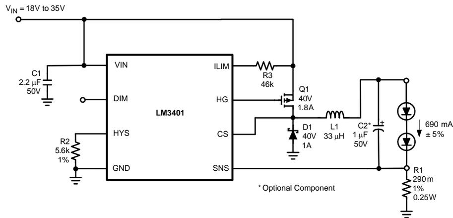
Figure 24. Example Circuit
