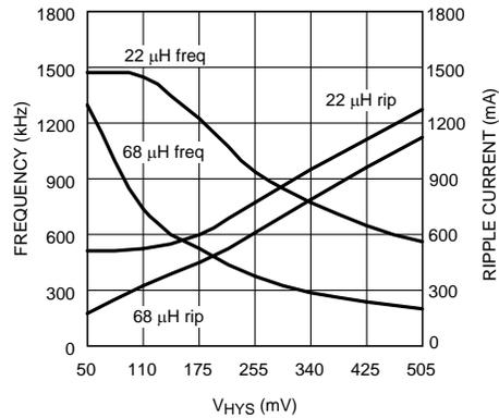
Figure 16. Switching Frequency and Ripple Current vs Hysteresis
