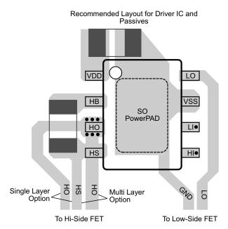
Figure 26. Recommended Layout Pattern
