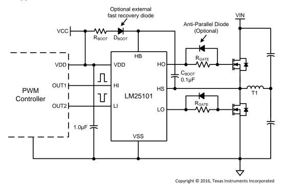
Figure 21. Application Diagram
