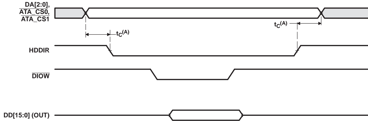
Figure 6-38. ATA/CF HDDIR Taskfile Write/Single PIO Write Timing
