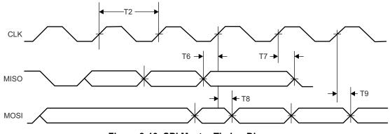
Figure 8-13. SPI Master Timing Diagram
