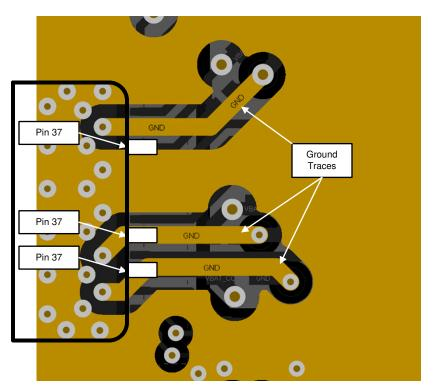
Figure 10-10. Ground Returns for Input Capacitors
