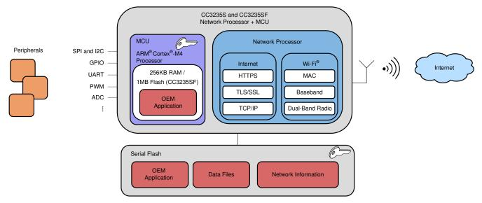
Figure 9-1. CC3235S and CC3235SF High-Level Structure
