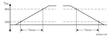
Figure 8-17. GPIO Timing Diagram
