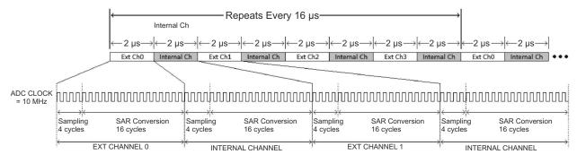
Figure 8-20. ADC Clock Timing Diagram
