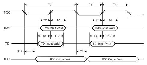
Figure 8-19. JTAG Timing Diagram
