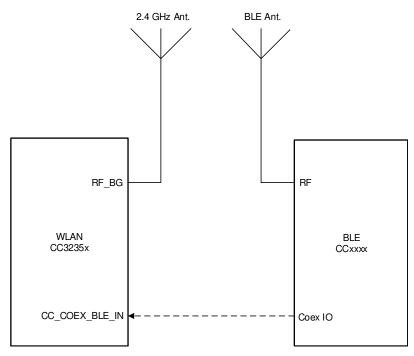
Figure 10-3. Dual-Antenna Coexistence Mode Block Diagram
