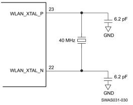
A. The crystal capacitance must be tuned to ensure that the PPM requirement is met. See CC31xx & CC32xx Frequency Tuning for information on frequency tuning.
