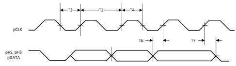
Figure 8-21. Camera Parallel Port Timing Diagram
