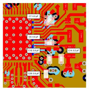
Figure 10-9. Ground Routing for Input Decoupling Capacitors
