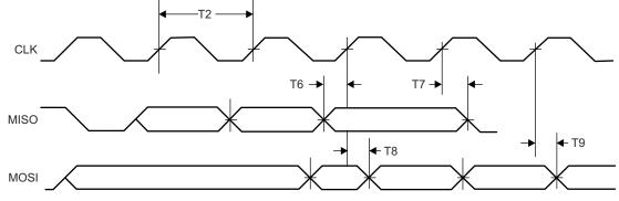
Figure 8-14. SPI Slave Timing Diagram
