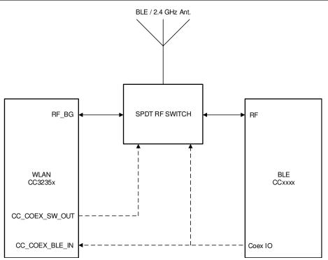
Figure 10-1. 2.4 GHz, Single-Antenna Coexistence Mode Block Diagram
