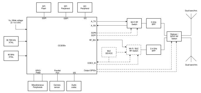
Note: The diplexer is used for the signal antenna solution. When using the antenna selection feature (dual antenna), an SPDT switch and 2 GPIO lines are required after the diplexer.
