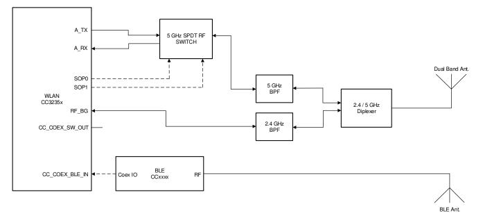
Figure 10-4. Dual Antenna Coexistence Solution with 5 GHz Wi-Fi
