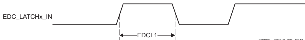
Figure 5-69. PRU-ICSS ECAT LATCHx_IN Timing
