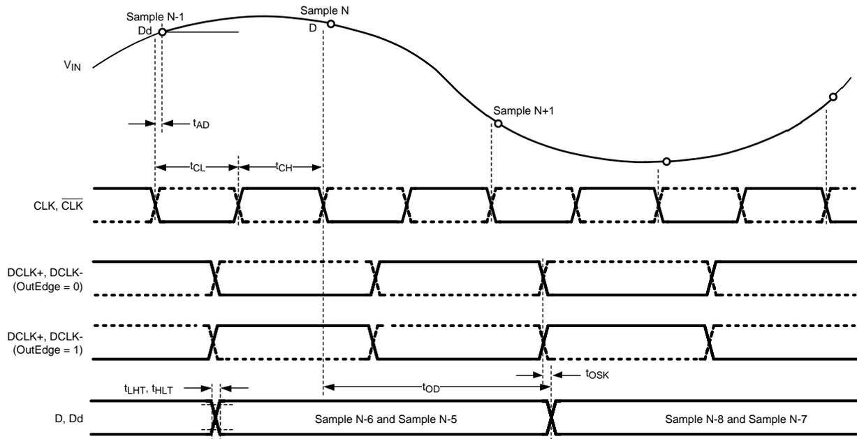
Figure 3. ADC081000 Timing
