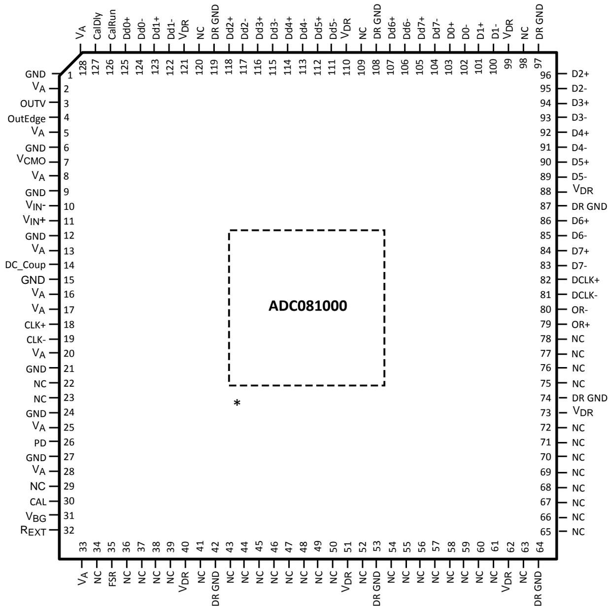
\* Exposed pad on back of package must be soldered to ground plane to ensure rated performance.
