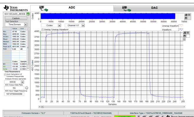
Figure 186. 40-MHz, Square-Wave Time Domain for 5-GSPS, Single-Channel Oscilloscope
