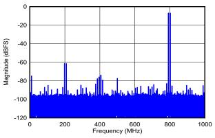
DES\_EN = 1,  $f_S$  = 2000MHz, FG calibration,  $f_1$  = 792MHz,  $f_2$ = 802MHz, A<sub>IN</sub> = -7dBFS per tone, SFDR = -62dBFS, IMD3 = -84dBFS, IMD2 = -74dBFS
