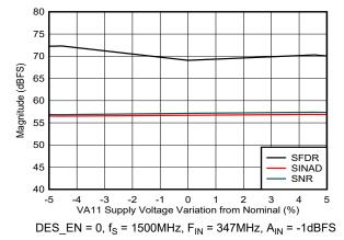
Figure 5-164. Performance vs VA11 Supply Voltage
