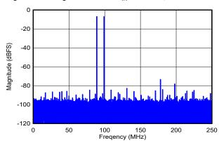
DES\_EN = 0,  $f_S$  = 500MHz, FG calibration,  $f_1$  = 89MHz,  $f_2$  = 99MHz,  $A_{IN}$  = -7dBFS per tone, SFDR = -73dBFS, IMD3 = -85dBFS, IMD2 = -92dBFS
