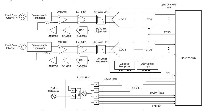
Figure 7-1. Typical Configuration for a Reconfigurable Oscilloscope
