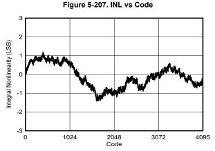
DES\_EN = 1,  $f_S$  = 4000MHz, FG calibration,  $F_{IN}$  = 99MHz
