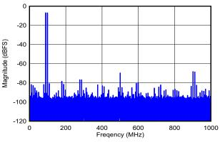
DES\_EN = 1,  $f_S$  = 2000MHz, FG calibration,  $f_1$  = 89MHz,  $f_2$  = 99MHz,  $A_{IN}$  = -7dBFS per tone, SFDR = -68dBFS, IMD3 = -81dBFS, IMD2 = -82dBFS
