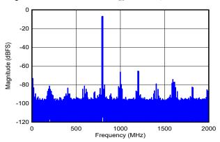
DES\_EN = 1,  $f_S$  = 4000MHz, FG calibration,  $f_1$  = 792MHz,  $f_2$  = 802MHz,  $A_{IN}$  = -7dBFS per tone, SFDR = -65dBFS, IMD3 = -87dBFS, IMD2 = -74dBFS
