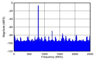
DES\_EN = 1,  $f_S$  = 5000MHz, FG calibration,  $f_1$  = 792MHz,  $f_2$  = 802MHz,  $A_{IN}$  = -7dBFS per tone, SFDR = -76dBFS, IMD3 = -93dBFS, IMD2 = -77dBFS
