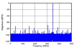
DES\_EN = 0, f<sub>S</sub> = 1000MHz, FG calibration, SNR = 57.8dBFS, SFDR = 68.5dBFS, ENOB = 9.1 bits
