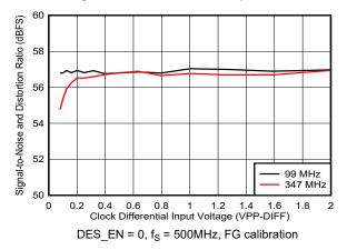
Figure 5-32. SINAD vs Clock Amplitude
