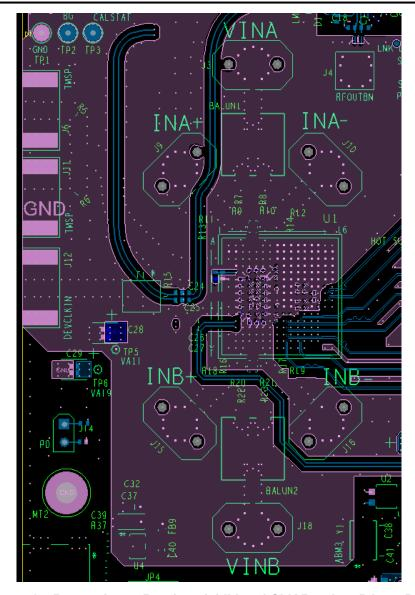
Figure 7-14. Bottom Layer Routing: Additional CLK Routing, DA4-7, DB4-7
