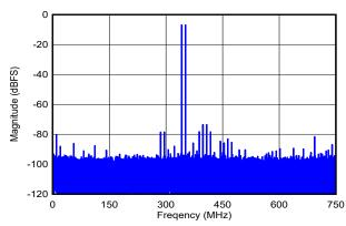
DES\_EN = 0,  $f_S$  = 1500MHz, FG calibration,  $f_1$  = 342MHz,  $f_2$  = 352MHz,  $A_{IN}$  = -7dBFS per tone, SFDR = -74dBFS, IMD3 = -92dBFS, IMD2 = -81dBFS
