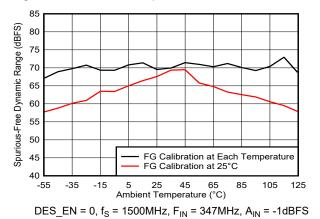
Figure 5-158. SFDR vs Temperature and Calibration Mode
