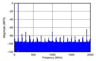
DES\_EN = 1,  $f_S$  = 4000MHz, FG calibration, SNR = 57.3dBFS, SFDR = 64.4dBFS, ENOB = 9.0 bits
