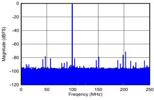
DES\_EN = 0,  $f_S$  = 500MHz, FG calibration, SNR = 57.5dBFS, SFDR = 71.4dBFS, ENOB = 9.2 bits
