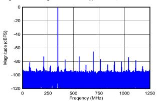
DES\_EN = 0,  $f_S$  = 2500MHz, FG calibration, SNR = 56.7dBFS. SFDR = 65.7dBFS. ENOB = 9.0 bits
