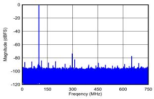
DES\_EN = 0, f<sub>S</sub> = 1500MHz, FG calibration, SNR = 57.5dBFS, SFDR = 73.8dBFS, ENOB = 9.2 bits
