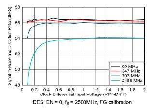
Figure 5-240. SINAD vs Clock Amplitude
