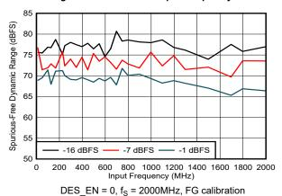
Figure 5-186. SFDR vs Input Frequency
