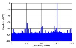
DES\_EN = 1, f<sub>S</sub> = 4000MHz, FG calibration, SNR = 56.2dBFS, SFDR = 61.8dBFS, ENOB = 8.6 bits
