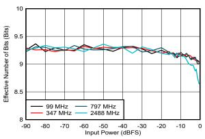
DES EN = 1,  $f_S$  = 3000MHz, FG calibration
