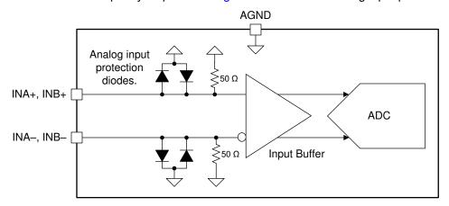
Figure 6-1. ADC12Dx500 Analog Input Internal Termination
