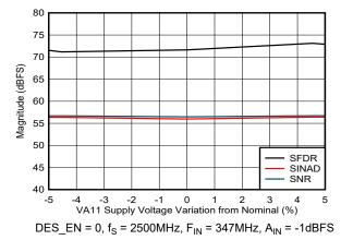
Figure 5-280. Performance vs VA11 Supply Voltage
