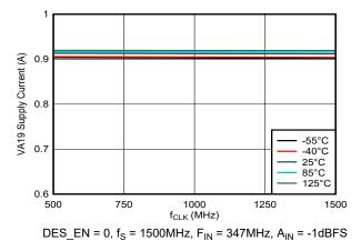
Figure 5-170. VA19 Supply Current vs Clock Rate
