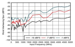
DES\_EN = 1,  $f_S$  = 5000MHz, FG calibration, includes  $f_S$  / 2 –  $f_{IN}$  and  $f_S$  /4 ±  $f_{IN}$  spurs only
