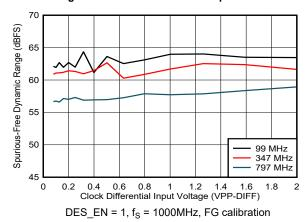
Figure 5-37. SFDR vs Clock Amplitude
