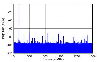
DES\_EN = 1, f<sub>S</sub> = 3000MHz, FG calibration, SNR = 57.4dBFS, SFDR = 71.3dBFS, ENOB = 9.0 bits
