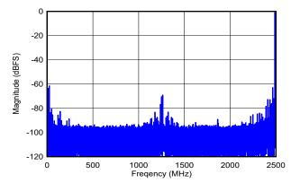
DES\_EN = 1, f<sub>S</sub> = 5000MHz, FG calibration, SNR = 55.7dBFS, SFDR = 61.5dBFS, ENOB = 8.5 bits
