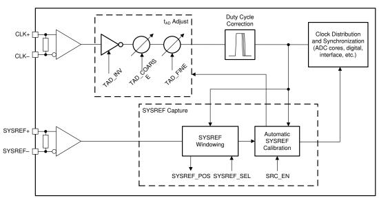
Figure 6-2. ADC12DLx500 Clocking Subsystem
