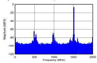
DES\_EN = 1,  $f_S$  = 4000MHz, FG calibration,  $f_1$  = 2483MHz,  $f_2$  = 2493MHz,  $A_{IN}$  = -7dBFS per tone, SFDR = -65dBFS, IMD3 = -73dBFS, IMD2 = -73dBFS
