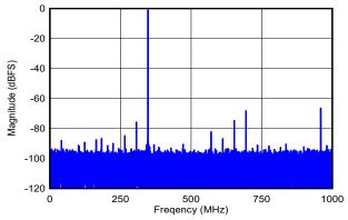
DES\_EN = 0, f<sub>S</sub> = 2000MHz, FG calibration, SNR = 57.3dBFS, SFDR = 66.4dBFS, ENOB = 9.0 bits
