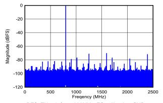
DES\_EN = 1,  $f_S$  = 5000MHz, FG calibration, SNR = 57.1dBFS, SFDR = 70.2dBFS, ENOB = 9.0 bits
