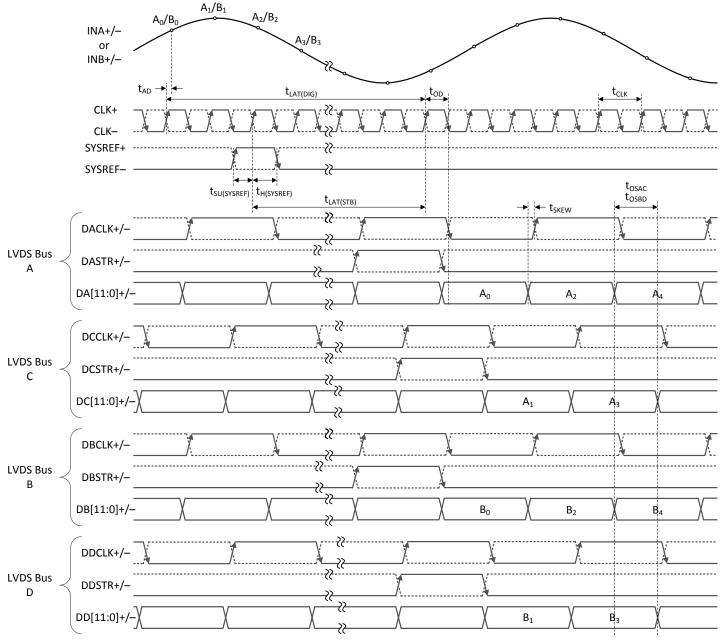
$t_{SU(SYSREF)}$  and  $t_{H(SYSREF)}$  are only shown for completeness. Use automatic SYSREF calibration or SYSREF windowing to meet SYSREF timing.
