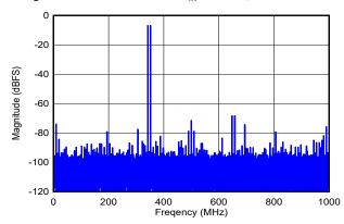
DES\_EN = 1,  $f_S$  = 2000MHz, FG calibration,  $f_1$  = 342MHz,  $f_2$  = 352MHz,  $A_{IN}$  = -7dBFS per tone, SFDR = -68dBFS, IMD3 = -89dBFS, IMD2 = -74dBFS
