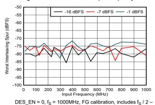
f<sub>IN</sub> spur only Figure 5-80. Worst Interleaving Spur vs Input Frequency
