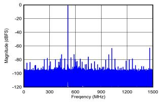
DES\_EN = 1, f<sub>S</sub> = 3000MHz, FG calibration, SNR = 56.2dBFS, SFDR = 62.8dBFS, ENOB = 8.7 bits
