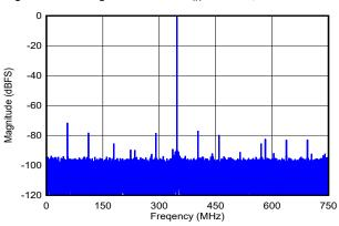
DES\_EN = 0, f<sub>S</sub> = 1500MHz, FG calibration, SNR = 57.6dBFS, SFDR = 71.7dBFS, ENOB = 9.2 bits
