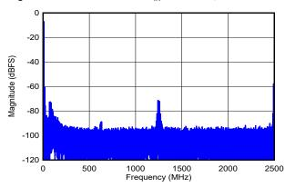
DES\_EN = 1,  $f_S$  = 5000MHz, FG calibration,  $f_1$  = 4992MHz,  $f_2$  = 5002MHz,  $A_{IN}$  = -7dBFS per tone, SFDR = -58dBFS, IMD3 = -61dBFS, IMD2 = -78dBFS
