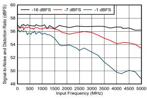
DES\_EN = 1,  $f_S$  = 5000MHz, FG calibration Figure 5-213. SINAD vs Input Frequency
