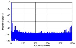
DES\_EN = 0, f<sub>S</sub> = 2500MHz, FG calibration, SNR = 55.2dBFS, SFDR = 64.6dBFS, ENOB = 8.7 bits
