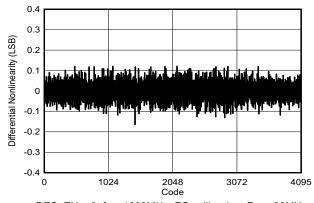
DES\_EN = 0,  $f_S$  = 1000MHz, FG calibration,  $F_{IN}$  = 99MHz
