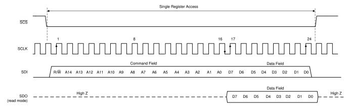
Figure 6-5. Serial Interface Protocol: Single Read/Write Operation
