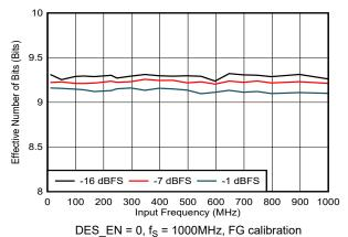
Figure 5-74. ENOB vs Input Frequency
