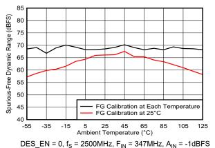
Figure 5-274. SFDR vs Temperature and Calibration Mode
