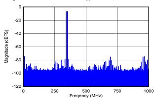
DES\_EN = 0,  $f_S$  = 2000MHz, FG calibration,  $f_1$  = 342MHz,  $f_2$  = 352MHz,  $A_{IN}$  = -7dBFS per tone, SFDR = -75dBFS, IMD3 = -79dBFS, IMD2 = -75dBFS
