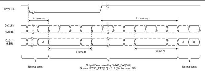
Figure 5-8. SYNCSE Timing Diagram
