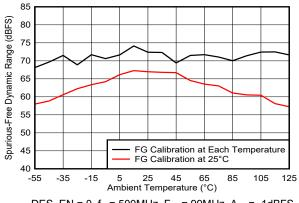
DES\_EN = 0,  $f_S$  = 500MHz,  $F_{IN}$  = 99MHz,  $A_{IN}$  = -1dBFS Figure 5-58. SFDR vs Temperature and Calibration Mode
