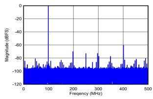
DES\_EN = 1, f<sub>S</sub> = 1000MHz, FG calibration, SNR = 57.1dBFS, SFDR = 60.5dBFS, ENOB = 8.8 bits
