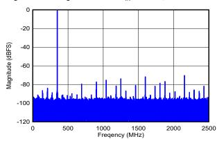
DES\_EN = 1,  $f_S$  = 5000MHz, FG calibration, SNR = 57.3dBFS, SFDR = 70.1dBFS, ENOB = 9.1 bits
