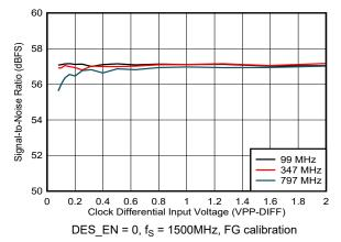
Figure 5-126. SNR vs Clock Amplitude
