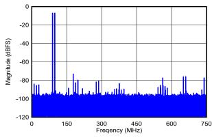
DES\_EN = 0,  $f_S$  = 1500MHz, FG calibration,  $f_1$  = 89MHz,  $f_2$  = 99MHz,  $A_{IN}$  = -7dBFS per tone, SFDR = -73dBFS, IMD3 = -98dBFS, IMD2 = -83dBFS
