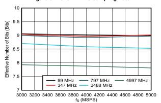
DES\_EN = 1, f<sub>S</sub> = 5000MHz, FG calibration
