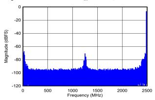
DES\_EN = 1,  $f_S$  = 5000MHz, FG calibration,  $f_1$  = 2483MHz,  $f_2$  = 2493MHz,  $A_{IN}$  = -7dBFS per tone, SFDR = -67dBFS, IMD3 = -74dBFS, IMD2 = -73dBFS
