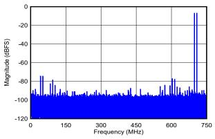
DES\_EN = 0,  $f_S$  = 1500MHz, FG calibration,  $f_1$  = 792MHz,  $f_2$  = 802MHz,  $A_{IN}$  = -7dBFS per tone, SFDR = -74dBFS, IMD3 = -90dBFS, IMD2 = -82dBFS
