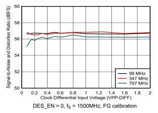
Figure 5-128. SINAD vs Clock Amplitude
