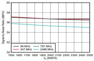
DES EN = 0, f<sub>S</sub> = 2500MHz, FG calibration
