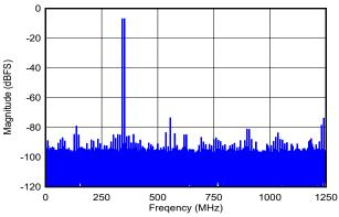
DES\_EN = 0,  $f_S$  = 2500MHz, FG calibration,  $f_1$  = 342MHz,  $f_2$  = 352MHz,  $A_{IN}$  = -7dBFS per tone, SFDR = -74dBFS, IMD3 = -86dBFS, IMD2 = -88dBFS
