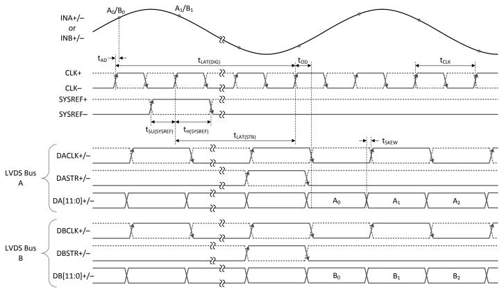
$t_{SU(SYSREF)}$  and  $t_{H(SYSREF)}$  are only shown for completeness. Use automatic SYSREF calibration or SYSREF windowing to meet SYSREF timing.
