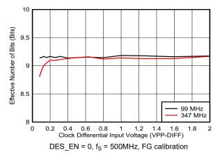
Figure 5-34. ENOB vs Clock Amplitude
