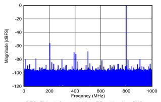
DES\_EN = 1,  $f_S$  = 2000MHz, FG calibration, SNR = 57.3dBFS, SFDR = 56.0dBFS, ENOB = 8.5 bits
