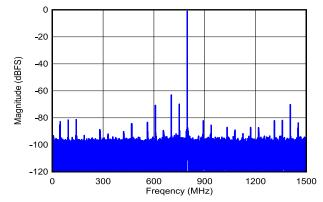
DES\_EN = 1,  $f_S$  = 3000MHz, FG calibration, SNR = 57.3dBFS, SFDR = 62.8dBFS, ENOB = 8.9 bits
