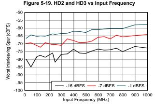
DES\_EN = 1,  $f_S$  = 1000MHz, FG calibration, includes  $f_S$  / 2 –  $f_{IN}$  and  $f_S$  /4 ±  $f_{IN}$  spurs only
