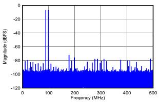
DES\_EN = 0,  $f_S$  = 1000MHz, FG calibration,  $f_1$  = 89MHz,  $f_2$  = 99MHz,  $A_{IN}$  = -7dBFS per tone, SFDR = -72dBFS, IMD3 = -85dBFS, IMD2 = -81dBFS
