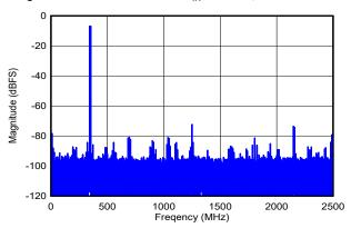
DES\_EN = 1,  $f_S$  = 5000MHz, FG calibration,  $f_1$  = 342MHz,  $f_2$  = 352MHz,  $A_{IN}$  = -7dBFS per tone, SFDR = -74dBFS, IMD3 = -91dBFS, IMD2 = -80dBFS
