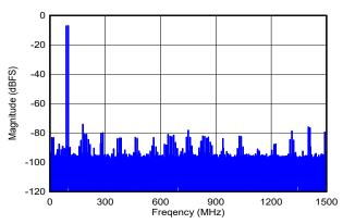
DES\_EN = 1,  $f_S$  = 3000MHz, FG calibration,  $f_1$  = 89MHz,  $f_2$  = 99MHz,  $A_{IN}$  = -7dBFS per tone, SFDR = -74dBFS, IMD3 = -90dBFS, IMD2 = -82dBFS
