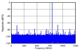
DES\_EN = 0,  $f_S$  = 2500MHz, FG calibration, SNR = 56.8dBFS, SFDR = 65.8dBFS, ENOB = 9.0 bits
