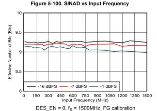
Figure 5-102. ENOB vs Input Frequency
