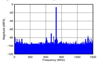
DES\_EN = 1,  $f_S$  = 3000MHz, FG calibration,  $f_1$  = 792MHz,  $f_2$  = 802MHz,  $A_{\text{IN}}$  = -7dBFS per tone, SFDR = -71dBFS, IMD3 = -84dBFS, IMD2 = -77dBFS
