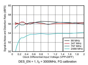
Figure 5-129. SINAD vs Clock Amplitude
