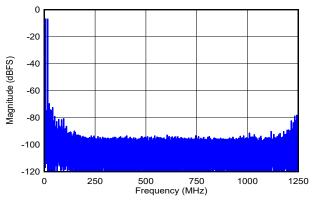
DES\_EN = 0,  $f_S$  = 2500MHz, FG calibration,  $f_1$  = 2483MHz,  $f_2$  = 2493MHz,  $A_{IN}$  = -7dBFS per tone, SFDR = -70dBFS, IMD3 = -76dBFS, IMD2 = -74dBFS
