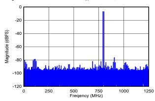
DES\_EN = 0,  $f_S$  = 2500MHz, FG calibration,  $f_1$  = 792MHz,  $f_2$  = 802MHz,  $A_{\text{IN}}$  = -7dBFS per tone, SFDR = -76dBFS, IMD3 = -91dBFS, IMD2 = -78dBFS
