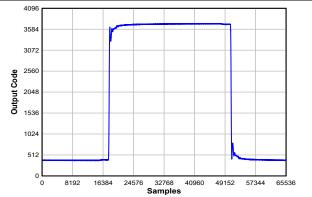
Figure 7-3. 50MHz, Unwrapped Square-Wave Time Domain for 5GSPS, Single-Channel Oscilloscope
