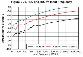
DES\_EN = 1,  $f_S$  = 2000MHz, FG calibration, includes  $f_S$  / 2 –  $f_{IN}$  and  $f_{S}$  /4 ±  $f_{IN}$  spurs only
