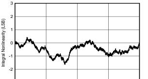
2048 Code DES\_EN = 1,  $f_S$  = 2000MHz, FG calibration,  $F_{IN}$  = 99MHz
