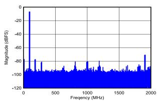
DES\_EN = 1,  $f_S$  = 4000MHz, FG calibration,  $f_1$  = 89MHz,  $f_2$  = 99MHz,  $A_{IN}$  = -7dBFS per tone, SFDR = -71dBFS, IMD3 = -94dBFS, IMD2 = -77dBFS
