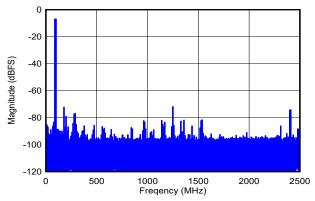
DES\_EN = 1,  $f_S$  = 5000MHz, FG calibration,  $f_1$  = 89MHz,  $f_2$  = 99MHz,  $A_{IN}$  = -7dBFS per tone, SFDR = -72dBFS, IMD3 = -86dBFS, IMD2 = -86dBFS
