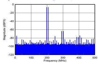
DES\_EN = 1,  $f_S$  = 1000MHz, FG calibration,  $f_1$  = 792MHz,  $f_2$  = 802MHz,  $A_{IN}$  = -7dBFS per tone, SFDR = -64dBFS, IMD3 = -87dBFS, IMD2 = -75dBFS
