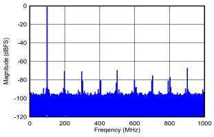
DES\_EN = 1,  $f_S$  = 2000MHz, FG calibration, SNR = 57.4dBFS, SFDR = 67.3dBFS, ENOB = 9.0 bits
