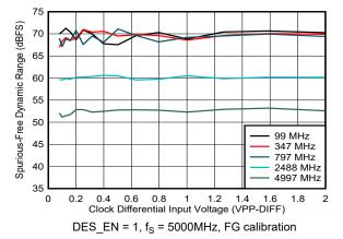
Figure 5-245. SFDR vs Clock Amplitude
