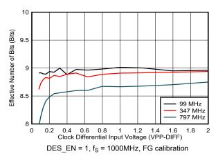
Figure 5-35. ENOB vs Clock Amplitude
