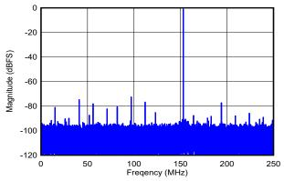
DES\_EN = 0,  $f_S$  = 500MHz, FG calibration, SNR = 57.5dBFS, SFDR = 72.5dBFS, ENOB = 9.2 bits
