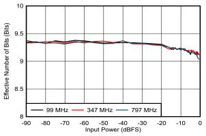
DES EN = 0,  $f_S = 1500MHz$ , FG calibration
