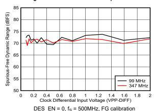
Figure 5-36. SFDR vs Clock Amplitude
