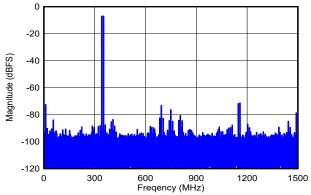
DES\_EN = 1,  $f_S$  = 3000MHz, FG calibration,  $f_1$  = 342MHz,  $f_2$  = 352MHz,  $A_{IN}$  = -7dBFS per tone, SFDR = -71dBFS, IMD3 = -88dBFS, IMD2 = -73dBFS
