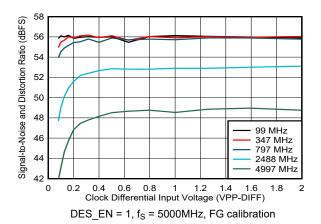
Figure 5-241. SINAD vs Clock Amplitude
