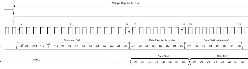
Figure 6-6. Serial Interface Protocol: Streaming Read/Write Operation
