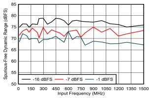
DES EN = 0, f<sub>S</sub> = 1500MHz, FG calibration
