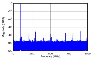
DES\_EN = 0, f<sub>S</sub> = 2000MHz, FG calibration, SNR = 57.3dBFS, SFDR = 70.6dBFS, ENOB = 9.1 bits
