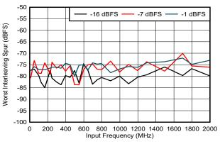
DES\_EN = 0,  $f_S$  = 2000MHz, FG calibration, includes  $f_S$  / 2 –  $f_{IN}$  spur only
