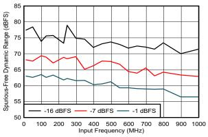
DES\_EN = 1, f<sub>S</sub> = 1000MHz, FG calibration
