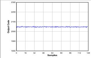
Figure 7-6. Idle-Channel Noise (No Input) for 5GSPS, Single-Channel Oscilloscope
