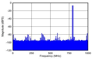
DES\_EN = 0,  $f_S$  = 2000MHz, FG calibration,  $f_1$  = 792MHz,  $f_2$  = 802MHz,  $A_{IN}$  = -7dBFS per tone, SFDR = -76dBFS, IMD3 = -88dBFS, IMD2 = -81dBFS
