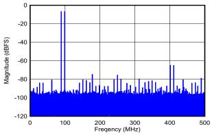
DES\_EN = 1,  $f_S$  = 1000MHz, FG calibration,  $f_1$  = 89MHz,  $f_2$  = 99MHz,  $A_{IN}$  = -7dBFS per tone, SFDR = -65dBFS, IMD3 = -95dBFS, IMD2 = -89dBFS
