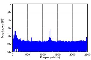
DES\_EN = 1, f<sub>S</sub> = 5000MHz, FG calibration, SNR = 53.2dBFS, SFDR = 53.2dBFS, ENOB = 7.9 bits
