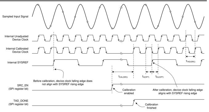
Figure 6-3. SYSREF Calibration Timing Diagram
