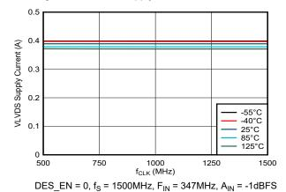
Figure 5-176. VLVDS Supply Current vs Clock Rate
