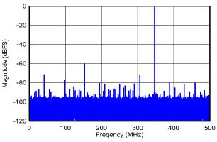
DES\_EN = 1, f<sub>S</sub> = 1000MHz, FG calibration, SNR = 57.3dBFS, SFDR = 60.0dBFS, ENOB = 8.8 bits
