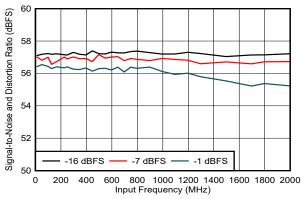
DES EN = 0,  $f_S = 2000MHz$ , FG calibration
