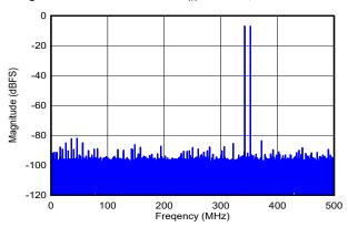
DES\_EN = 0,  $f_S$  = 1000MHz, FG calibration,  $f_1$  = 342MHz,  $f_2$  = 352MHz,  $A_{\text{IN}}$  = -7dBFS per tone, SFDR = -82dBFS, IMD3 = -96dBFS, IMD2 = -89dBFS
