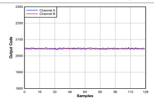
Figure 7-9. Idle-Channel Noise (No Input) for 2.5GSPS, Dual-Channel Oscilloscope
