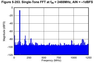
DES\_EN = 0,  $f_S$  = 2500MHz, FG calibration,  $f_1$  = 89MHz,  $f_2$  = 99MHz,  $A_{\text{IN}}$  = -7dBFS per tone, SFDR = -71dBFS, IMD3 = -86dBFS, IMD2 = -71dBFS
