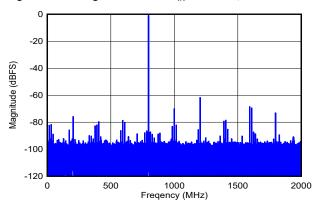
DES\_EN = 1, f<sub>S</sub> = 4000MHz, FG calibration, SNR = 57.1dBFS, SFDR = 61.7dBFS, ENOB = 8.8 bits
