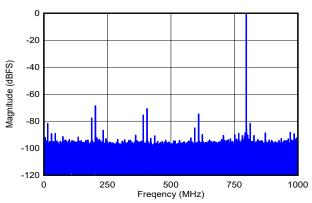
DES\_EN = 0, f<sub>S</sub> = 2000MHz, FG calibration, SNR = 57.0dBFS, SFDR = 68.5dBFS, ENOB = 9.1 bits
