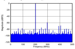
DES\_EN = 1, f<sub>S</sub> = 1000MHz, FG calibration, SNR = 57.1dBFS, SFDR = 59.0dBFS, ENOB = 8.7 bits
