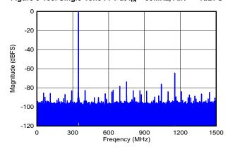
DES\_EN = 1,  $f_S$  = 3000MHz, FG calibration, SNR = 57.6dBFS, SFDR = 64.2dBFS, ENOB = 9.1 bits
