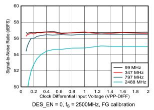
Figure 5-238. SNR vs Clock Amplitude
