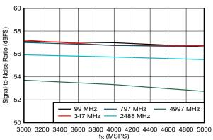
DES\_EN = 1, f<sub>S</sub> = 5000MHz, FG calibration
