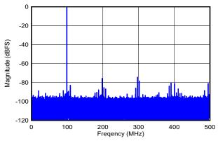
DES\_EN = 0, f<sub>S</sub> = 1000MHz, FG calibration, SNR = 57.5dBFS, SFDR = 74.4dBFS, ENOB = 9.2 bits
