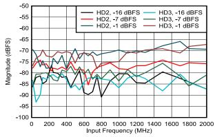
DES EN = 0, f<sub>S</sub> = 2000MHz, FG calibration
