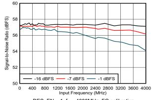
DES\_EN = 1, f<sub>S</sub> = 4000MHz, FG calibration Figure 5-181. SNR vs Input Frequency
