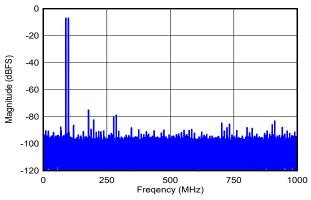
DES\_EN = 0,  $f_S$  = 2000MHz, FG calibration,  $f_1$  = 89MHz,  $f_2$  = 99MHz,  $A_{IN}$  = -7dBFS per tone, SFDR = -75dBFS, IMD3 = -95dBFS, IMD2 = -90dBFS
