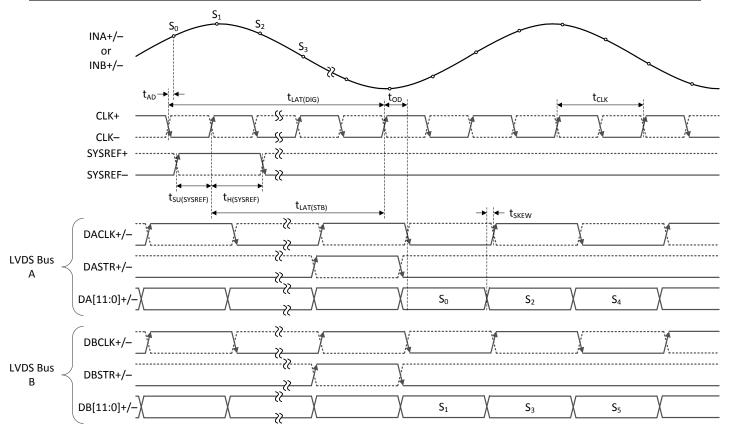
$t_{\text{SU(SYSREF})}$  and  $t_{\text{H(SYSREF})}$  are only shown for completeness. Use automatic SYSREF calibration or SYSREF windowing to meet SYSREF timing.
