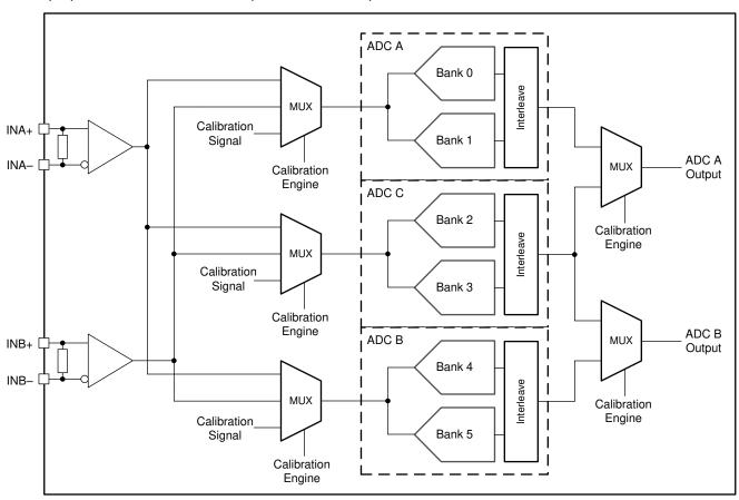
Figure 6-4. ADC12DLx500 Calibration System Block Diagram
