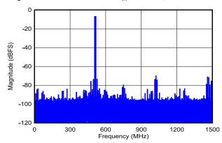
DES\_EN = 1,  $f_S$  = 3000MHz, FG calibration,  $f_1$  = 2483MHz,  $f_2$  = 2493MHz,  $A_{IN}$  = -7dBFS per tone, SFDR = -70dBFS, IMD3 = -74dBFS, IMD2 = -75dBFS
