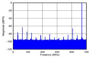
DES\_EN = 0,  $f_S$  = 1500MHz, FG calibration, SNR = 57.2dBFS, SFDR = 63.5dBFS, ENOB = 8.9 bits
