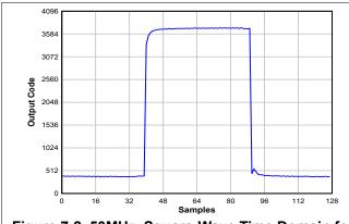
Figure 7-2. 50MHz, Square-Wave Time Domain for 5GSPS, Single-Channel Oscilloscope
