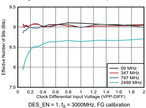
Figure 5-131. ENOB vs Clock Amplitude
