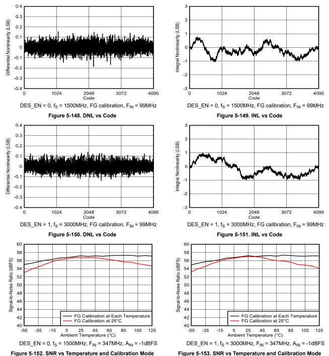
Figure 5-153. SNR vs Temperature and Calibration Mode
