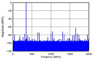
DES\_EN = 1,  $f_S$  = 4000MHz, FG calibration, SNR = 56.9dBFS, SFDR = 62.7dBFS, ENOB = 8.9 bits
