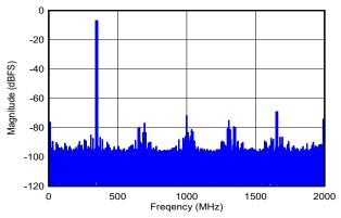
DES\_EN = 1,  $f_S$  = 4000MHz, FG calibration,  $f_1$  = 342MHz,  $f_2$  = 352MHz,  $A_{IN}$  = -7dBFS per tone, SFDR = -69dBFS, IMD3 = -95dBFS, IMD2 = -77dBFS
