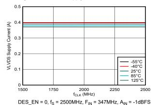
Figure 5-292. VLVDS Supply Current vs Clock Rate
