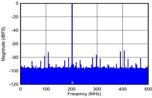
DES\_EN = 0, f<sub>S</sub> = 1000MHz, FG calibration, SNR = 57.3dBFS, SFDR = 69.8dBFS, ENOB = 9.1 bits
