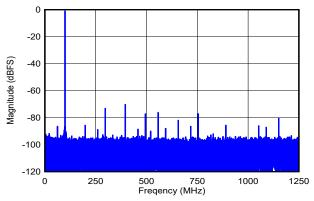
DES\_EN = 0, f<sub>S</sub> = 2500MHz, FG calibration, SNR = 57.1dBFS, SFDR = 70.3dBFS, ENOB = 9.1 bits
