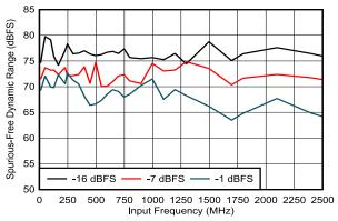
DES EN = 0,  $f_S = 2500MHz$ , FG calibration
