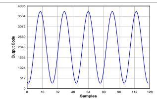
Figure 7-4. 200MHz, Sine-Wave Time Domain for 5GSPS, Single-Channel Oscilloscope
