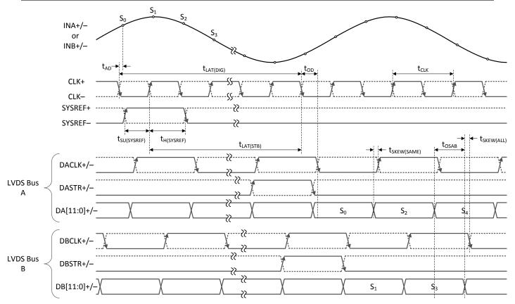
$t_{\text{SU(SYSREF})}$  and  $t_{\text{H(SYSREF})}$  are only shown for completeness. Use automatic SYSREF calibration or SYSREF windowing to meet SYSREF timing.
