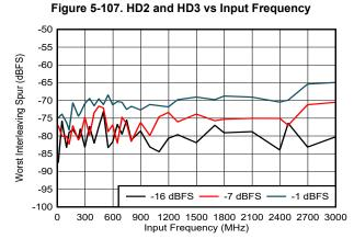
DES\_EN = 1,  $f_S$  = 3000MHz, FG calibration, includes  $f_S$  / 2 –  $f_{IN}$  and  $f_S$  /4 ±  $f_{IN}$  spurs only
