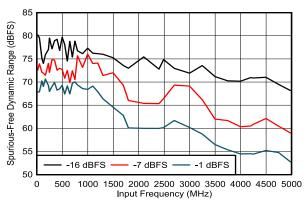
DES EN = 1,  $f_S$  = 5000MHz, FG calibration
