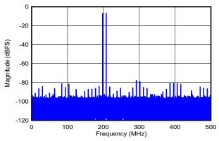
DES\_EN = 0,  $f_S$  = 1000MHz, FG calibration,  $f_1$  = 792MHz,  $f_2$ = 802MHz, A<sub>IN</sub> = -7dBFS per tone, SFDR = -78dBFS, IMD3 = -84dBFS, IMD2 = -85dBFS
