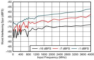
DES\_EN = 1,  $f_S$  = 4000MHz, FG calibration, includes  $f_S$  / 2 –  $f_{IN}$  and  $f_S$  /4 ±  $f_{IN}$  spurs only
