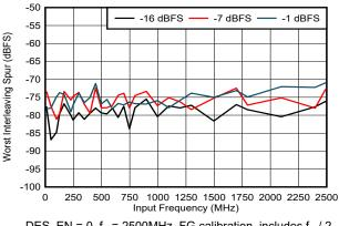
DES\_EN = 0,  $f_S$  = 2500MHz, FG calibration, includes  $f_S / 2 - f_{IN}$  spur only
