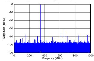
DES\_EN = 1,  $f_S$  = 2000MHz, FG calibration, SNR = 57.5dBFS, SFDR = 62.8dBFS, ENOB = 9.0 bits
