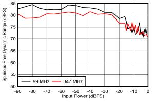
DES EN = 0,  $f_S = 500MHz$ , FG calibration
