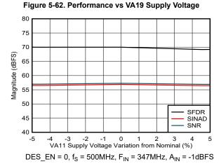
Figure 5-64. Performance vs VA11 Supply Voltage
