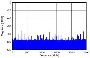
DES\_EN = 1,  $f_S$  = 5000MHz, FG calibration, SNR = 57.0dBFS, SFDR = 71.7dBFS, ENOB = 9.1 bits
