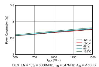
Figure 5-178. Power Consumption vs Clock Rate
