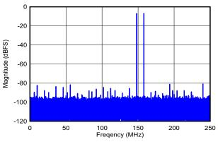
DES\_EN = 0,  $f_S$  = 500MHz, FG calibration,  $f_1$  = 342MHz,  $f_2$  = 352MHz,  $A_{IN}$  = -7dBFS per tone, SFDR = -81dBFS, IMD3 = -87dBFS, IMD2 = -82dBFS
