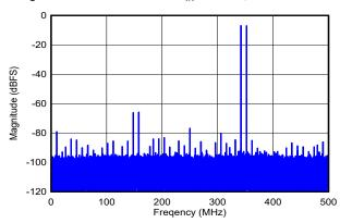
DES\_EN = 1,  $f_S$  = 1000MHz, FG calibration,  $f_1$  = 342MHz,  $f_2$  = 352MHz,  $A_{\text{IN}}$  = -7dBFS per tone, SFDR = -66dBFS, IMD3 = -85dBFS, IMD2 = -80dBFS
