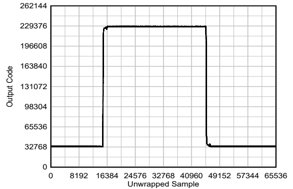
Unwrapped 1MHz Square Wave Figure 5-20. Pulse Response
