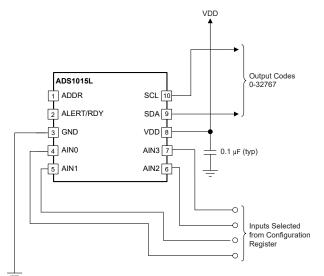
NOTE: Digital pin connections omitted for clarity.
