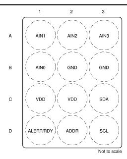
Figure 5-2. YCJ Package, 12-Pin DSBGA (Top View)
