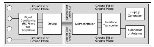
Figure 9-12. System Component Placement
