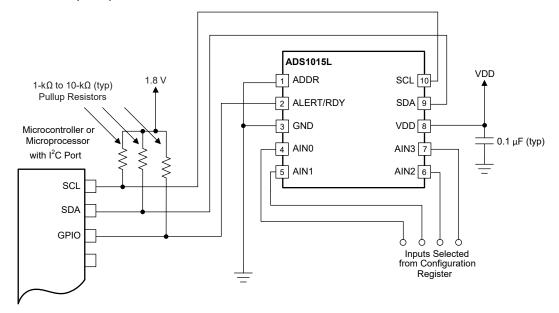
Figure 9-1. Typical Connections of the ADS1015L
