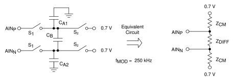
Figure 7-4. Simplified Analog Input Circuit
