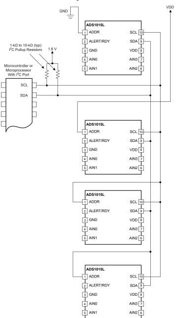
NOTE: The ADS101xL power and input connections are omitted for clarity. The ADDR pin selects the I<sup>2</sup>C address.
