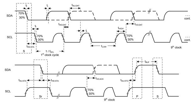
Figure 6-1. I<sup>2</sup>C Timing Requirements
