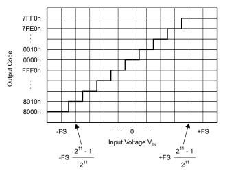
Figure 7-12. Code Transition Diagram
