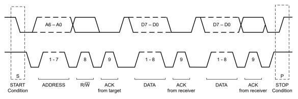
Figure 7-8. I<sup>2</sup>C Data Transfer Format
