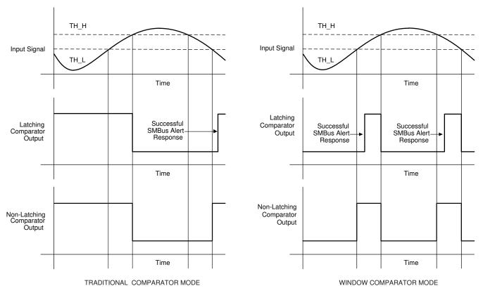
Figure 7-6. ALERT Pin Timing Diagram
