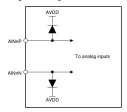
Figure 8-1. Input ESD Protection Circuitry
