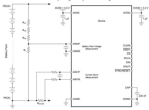
Figure 9-4. ADS131M08-Q1 in a Typical Battery Management System Application
