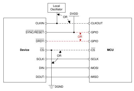
Figure 9-2. Minimum Connections Required to Operate the ADS131M08-Q1
