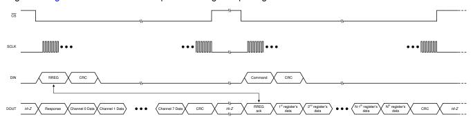
Figure 8-24. Reading Multiple Registers
