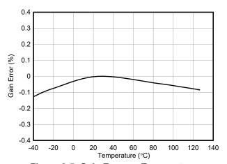
Figure 9-5. Gain Error vs Temperature
