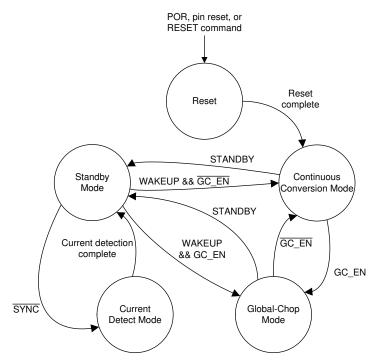
Figure 8-13. State Diagram Depicting Device Functional Modes
