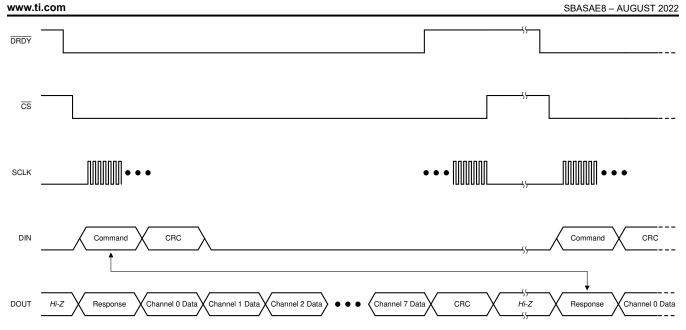
Figure 8-18. Typical Communication Frame
