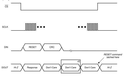
Figure 8-22. RESET Command Frame
