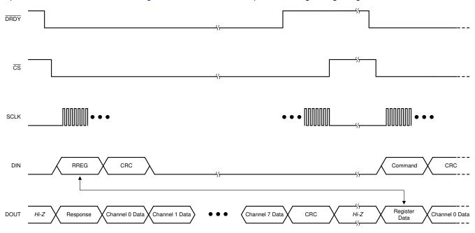
Figure 8-23. Reading a Single Register
