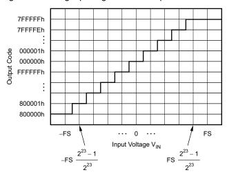
Figure 8-19. Code Transition Diagram
