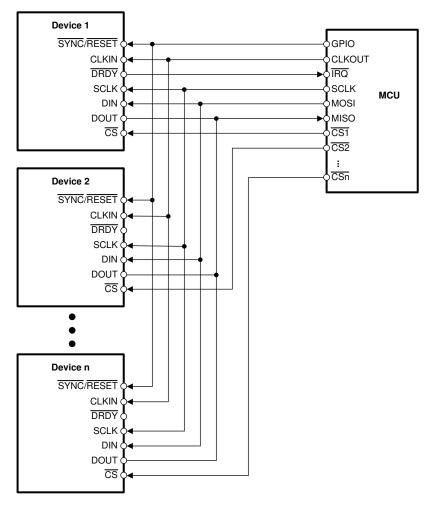
Figure 9-3. Multiple Device Configuration
