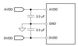
Figure 43. Power-Supply Decoupling
