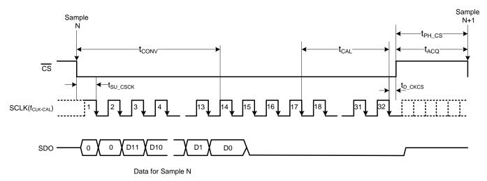
Figure 39. Offset Calibration During Normal Operation Timing Diagram
