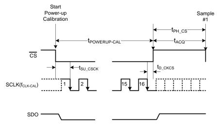
Figure 38. Offset Calibration on Power-Up Timing Diagram
