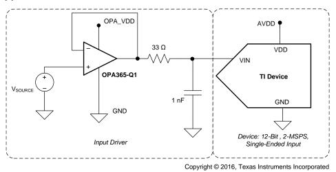
Figure 40. Single-Supply DAQ with the ADS7049-Q1
