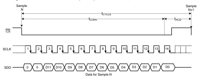
Figure 36. Serial Interface Timing Diagram
