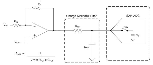
Figure 41. Charge Kickback Filter
