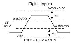
Figure 32. Digital Voltage Levels as per the JESD8-7A Standard
