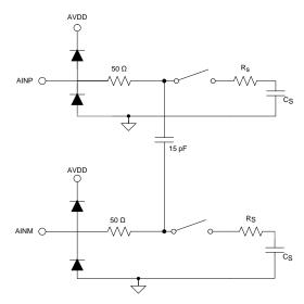
Figure 34. Equivalent Input Circuit for the Sampling Stage
