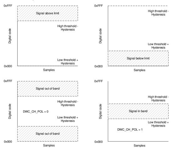
Figure 27. Event Monitoring With the Window Comparator
