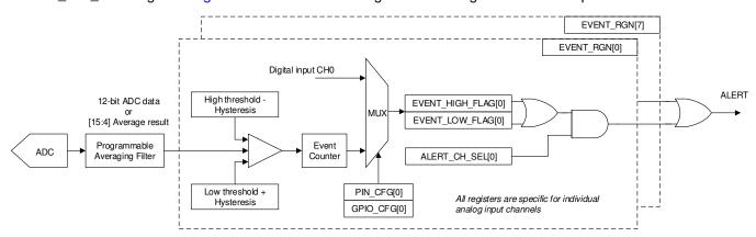
Figure 26. Digital Window Comparator Block Diagram
