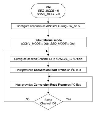
Manual mode with channel selection using register write
