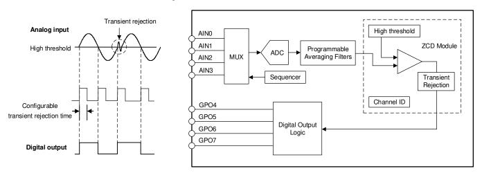
Figure 29. ZCD Module Operation Block Diagram
