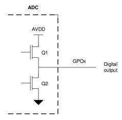
Figure 159. Digital Push-Pull Output
