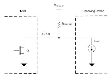
Figure 157. Digital Open-Drain Output
