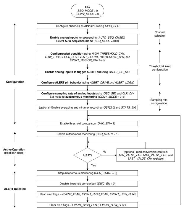
Figure 33. Configuring the Device in Autonomous Mode
