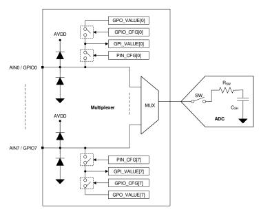
Figure 21. Analog Inputs, GPIOs, and ADC Connections
