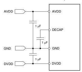
Figure 160. Power-Supply Decoupling
