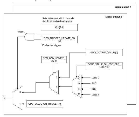
Figure 28. Block Diagram for the Digital Output Logic
