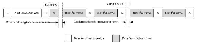
Figure 31. Starting a Conversion and Reading Data in Manual Mode
