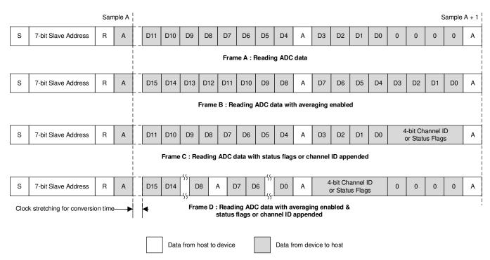
Figure 25. Data Frames for Reading Data
