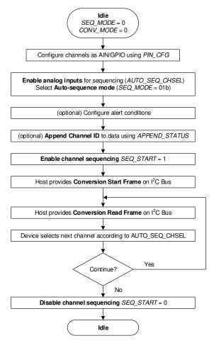
Figure 32. Device Operation in Auto-Sequence Mode
