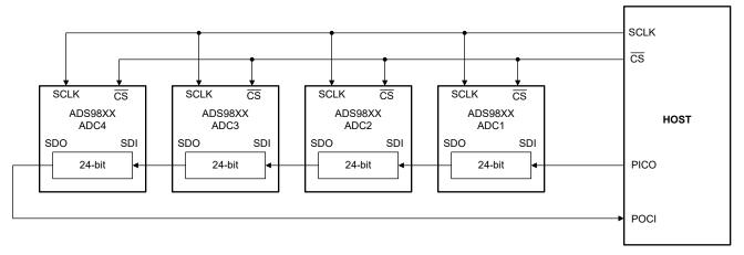
Figure 6-11. Daisy-Chain Connections for SPI Configuration
