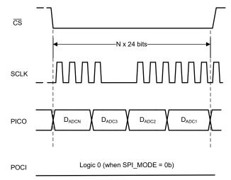
Figure 6-12. Register Write With Daisy-Chain
