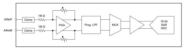
Figure 6-1. Front-End Circuit Schematic for the Selected Analog Input Channel
