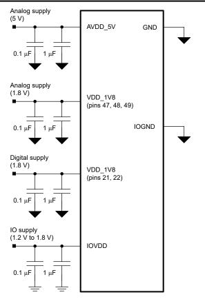
Figure 8-4. Power-Supply Decoupling
