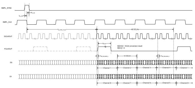
Figure 5-3. 2-SDO DDR CMOS Data Interface
