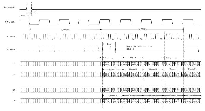
Figure 5-2. 4-SDO DDR CMOS Data Interface
