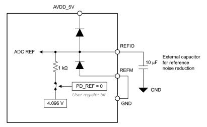
Figure 6-6. Internal Reference Voltage
