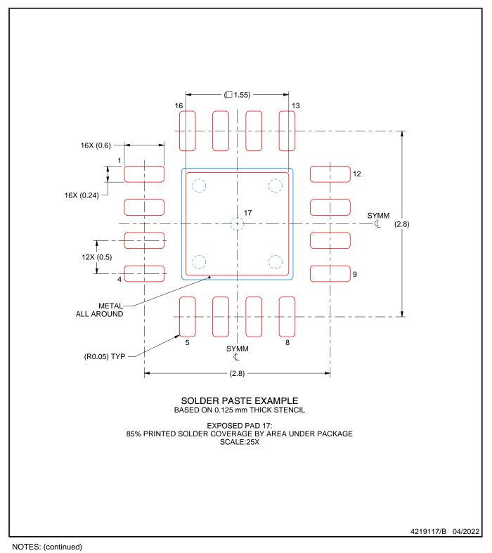
6. Laser cutting apertures with trapezoidal walls and rounded corners may offer better paste release. IPC-7525 may have alternate design recommendations.
