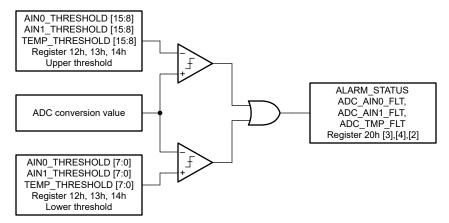
Figure 7-13. ADC Out-of-Range Alarm
