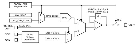
Figure 7-12. Alarm Voltage Generator Architecture
