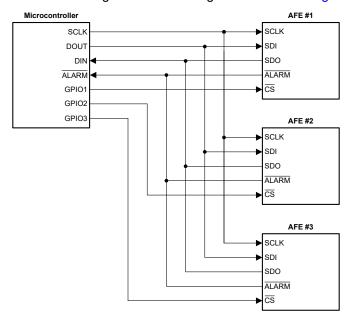
Figure 8-1. Multichannel Configuration
