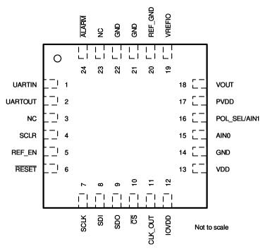
Figure 5-1. RRU (24-pin UQFN) Package, Top View
