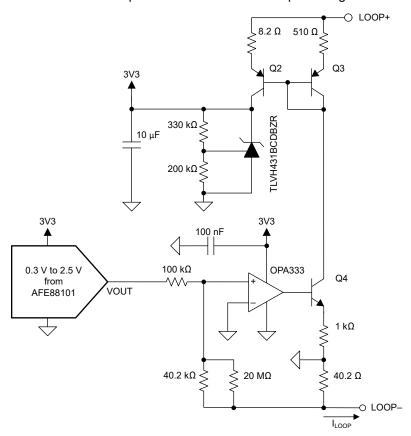
Figure 8-5. Current Loop Control for the AFE88101 Transmitter
