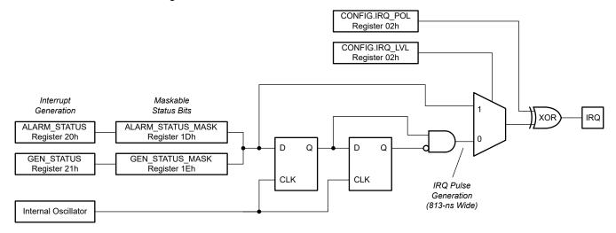
Figure 7-15. IRQ Block Diagram
