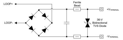
Figure 8-6. Loop Input Protection
