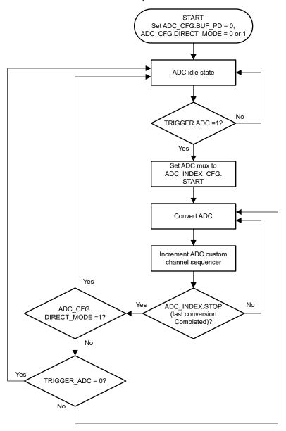
Figure 7-8. ADC Conversion Sequence
