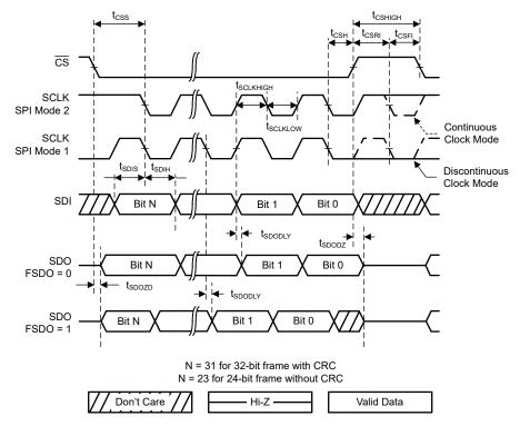
Figure 6-1. SPI Timing
