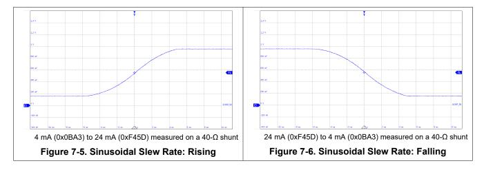
If the slew-rate feature is disabled while the DAC is executing the slew-rate command, the slew-rate operation is aborted, and the DAC output goes to the target code.
