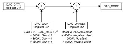
Figure 7-2. DAC Calibration Path
