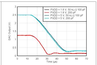
Figure 6-21. DAC Settling Time vs Load (Rising Voltage Step)
