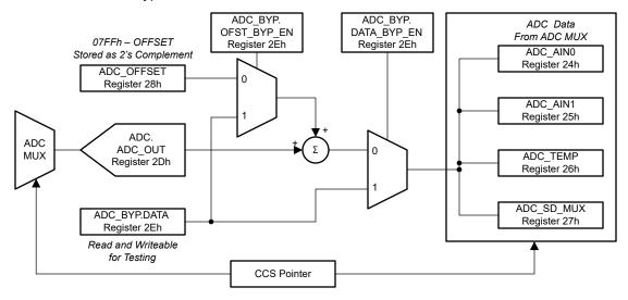
Figure 7-11. ADC Bypass Data Flow
