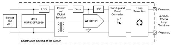
Figure 8-3. Block Diagram of a Loop-Powered, 4-mA to 20-mA Current Transmitter
