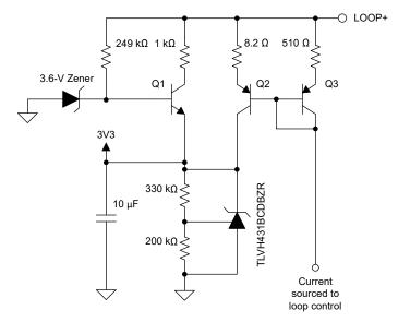
Figure 8-4. Start-Up Circuit
