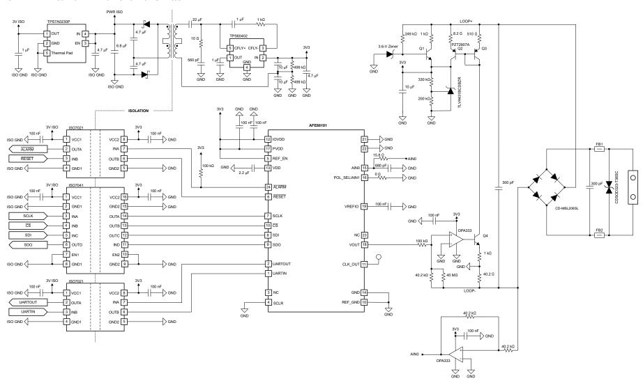
Figure 8-2. AFEx8101 in a 4-mA to 20-mA Current Transmitter
