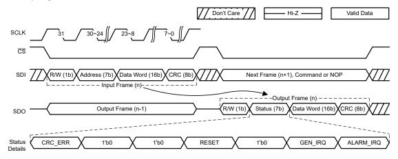
Figure 7-19. SPI Frame Details (Default, CRC Enabled)
