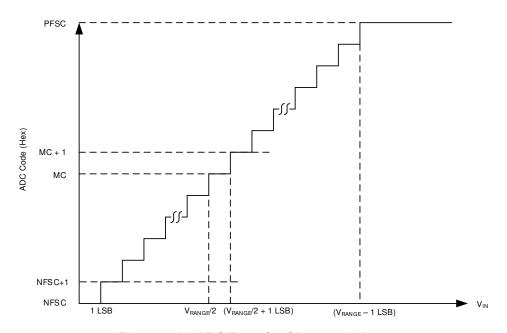
Figure 7-10. ADC Transfer Characteristics
