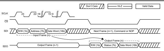
Figure 7-20. SPI Frame Details (CRC Disabled)
