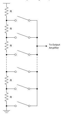
Figure 7-1. DAC Resistor String
