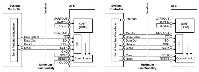
Figure 7-17. SPI Mode Connections
