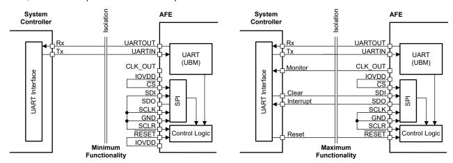
Figure 7-18. UBM (UART Interface) Connections
