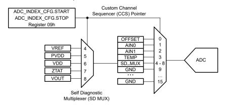
Figure 7-9. ADC MUX Control
