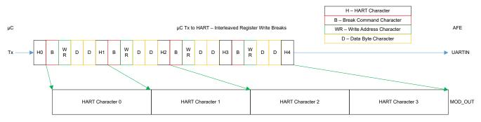
Figure 7-34. Interleaved HART Transmit With UBM Register Writes
