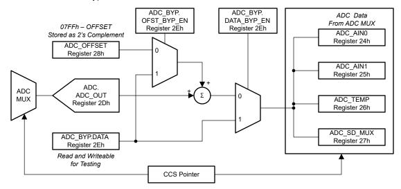
Figure 7-11. ADC Bypass Data Flow
