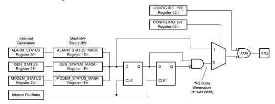
Figure 7-15. IRQ Block Diagram
