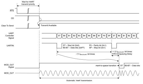
Figure 7-20. HART Transmit Start Timing Diagram (UART Mode)
