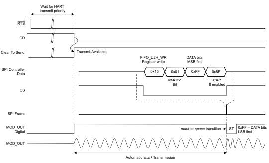
Figure 7-21. HART Transmit Start Timing Diagram (SPI Mode)
