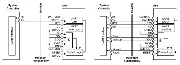
Figure 7-27. UBM (UART Interface) Connections
