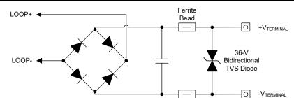
Figure 8-6. Loop Input Protection
