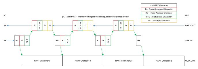
Figure 7-36. Interleaved HART Transmit With UBM Register Read Requests and Responses
