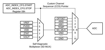
Figure 7-9. ADC MUX Control
