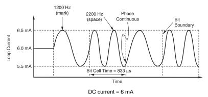
Figure 7-16. Output Current vs Time
