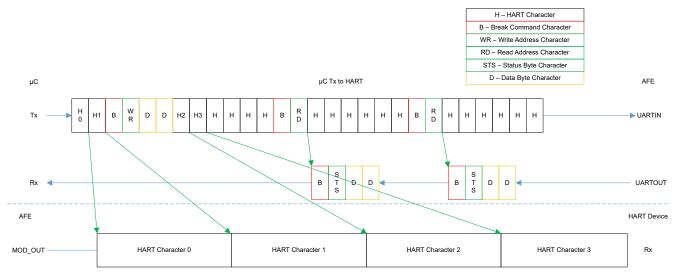
Figure 7-37. Packed HART Transmit With UBM Register Write and Read Requests and Responses
