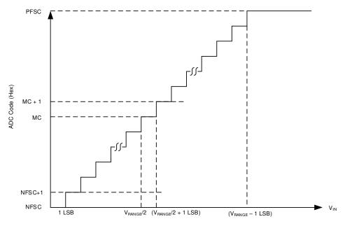
Figure 7-10. ADC Transfer Characteristics
