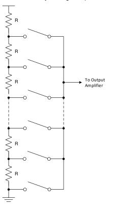
Figure 7-1. DAC Resistor String
