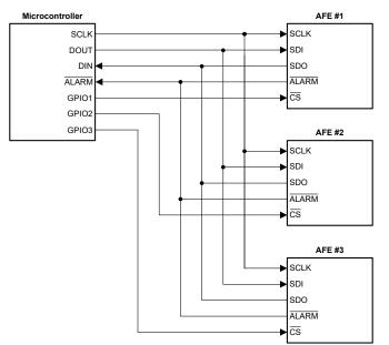
Figure 8-1. Multichannel Configuration
