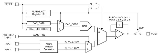
Figure 7-12. Alarm Voltage Generator Architecture
