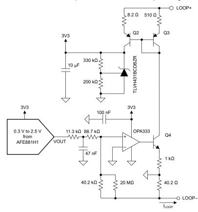
Figure 8-5. Current Loop Control for the AFE881H1 Transmitter
