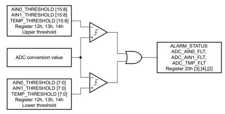
Figure 7-13. ADC Out-of-Range Alarm
