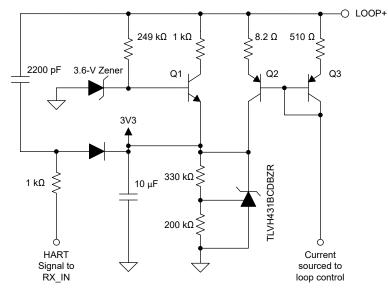
Figure 8-4. Start-Up Circuit
