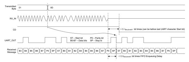
Figure 7-24. HART Receive End Timing Diagram (UART Mode)
