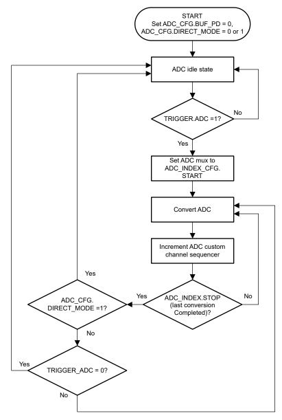
Figure 7-8. ADC Conversion Sequence
