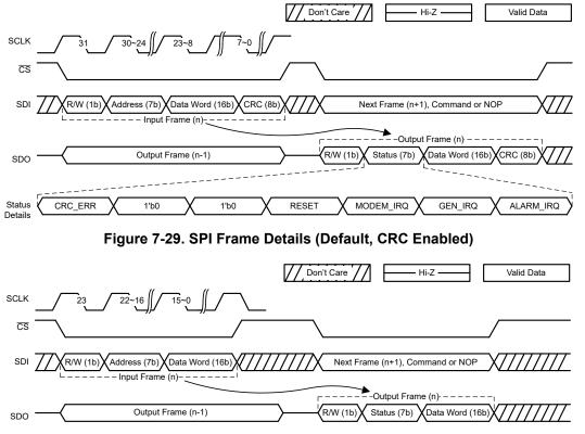
Figure 7-30. SPI Frame Details (CRC Disabled)
