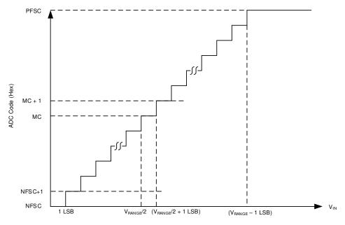
Figure 7-10. ADC Transfer Characteristics
