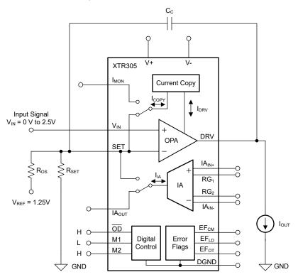
Figure 8-4. The XTR305 Standard Circuit for Current Output
