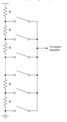
Figure 7-1. DAC Resistor String
