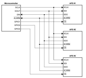
Figure 8-1. Multichannel Configuration
