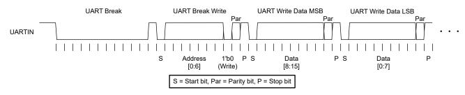
Figure 7-21. UARTIN Break Write Data Format
