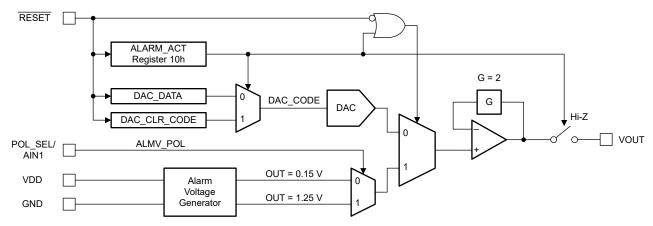
Figure 7-12. Alarm Voltage Generator Architecture
