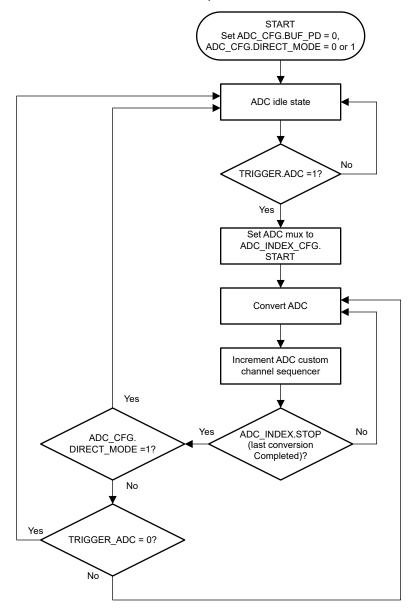
Figure 7-8. ADC Conversion Sequence
