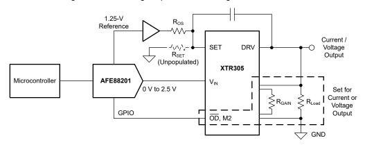
Figure 8-3. Block Diagram of the Analog Output Module Using the AFEx8201 and XTR305
