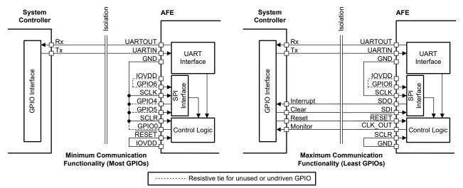
Figure 7-18. UBM (UART Interface) Connections
