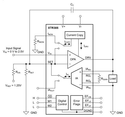
Figure 8-5. The XTR305 Standard Circuit for Voltage Output
