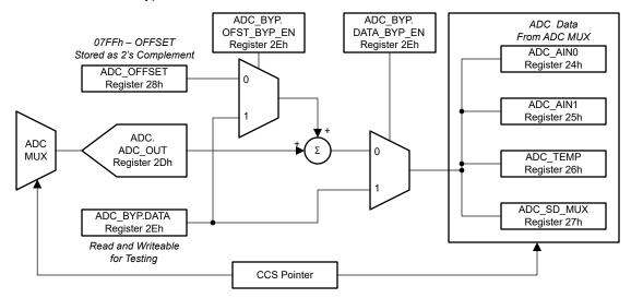
Figure 7-11. ADC Bypass Data Flow
