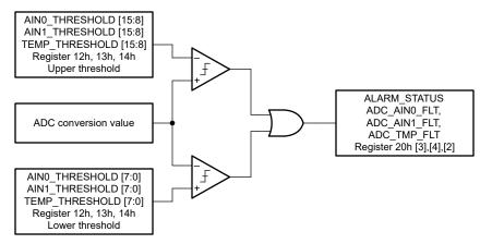
Figure 7-13. ADC Out-of-Range Alarm
