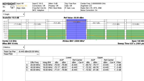
Figure 7-412. TX 20-MHz LTE Output Spectrum at 2.6 GHz (Band 41)
