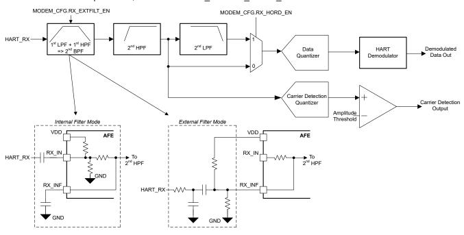
Figure 7-19. HART Demodulator Architecture
