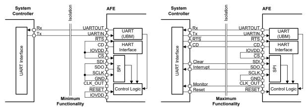
Figure 7-27. UBM (UART Interface) Connections
