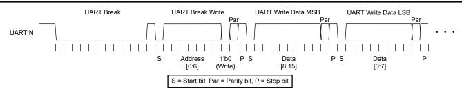
Figure 7-31. UARTIN Break Write Data Format
