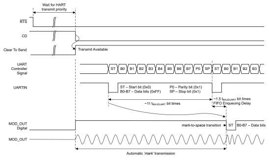
Figure 7-20. HART Transmit Start Timing Diagram (UART Mode)
