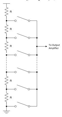
Figure 7-1. DAC Resistor String
