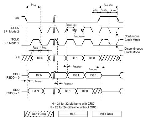
Figure 6-1. SPI Timing
