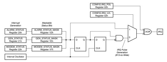
Figure 7-15. IRQ Block Diagram
