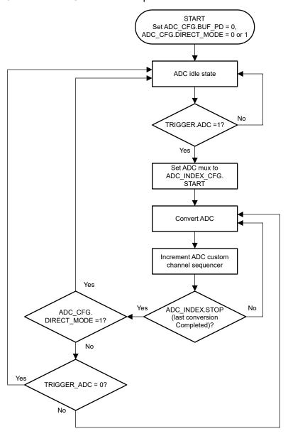
Figure 7-8. ADC Conversion Sequence
