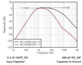
Figure 6-52. HART Internal Mode Complete Band-Pass Filter Response (From HART\_RX Signal to Internal Demodulator)
