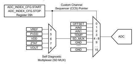
Figure 7-9. ADC MUX Control
