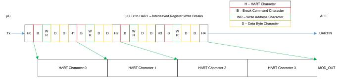
Figure 7-34. Interleaved HART Transmit With UBM Register Writes
