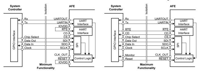
Figure 7-28. SPI Plus UART Mode Connections
