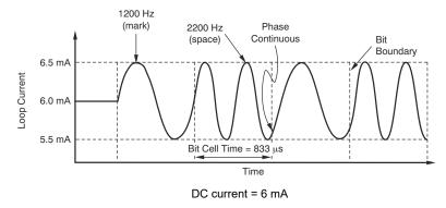
Figure 7-16. Output Current vs Time
