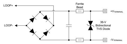
Figure 8-6. Loop Input Protection
