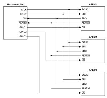
Figure 8-1. Multichannel Configuration
