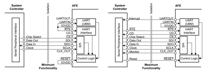
Figure 7-26. SPI Mode Connections
