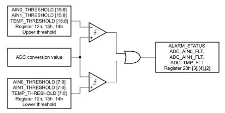
Figure 7-13. ADC Out-of-Range Alarm
