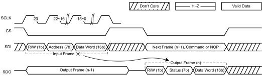
Figure 7-30. SPI Frame Details (CRC Disabled)
