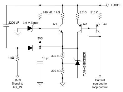
Figure 8-4. Start-Up Circuit
