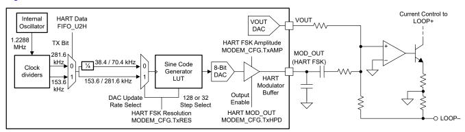
Figure 7-18. HART Modulator Architecture
