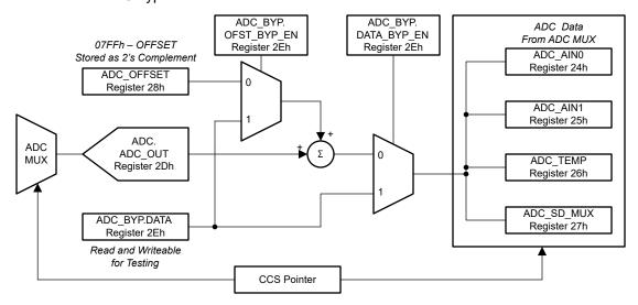
Figure 7-11. ADC Bypass Data Flow
