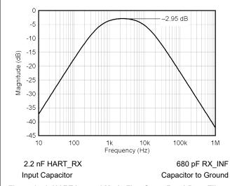
Figure 6-51. HART Internal Mode First Stage Band-Pass Filter Response (From HART\_RX Signal to RX\_INF Pin)
