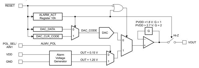
Figure 7-12. Alarm Voltage Generator Architecture
