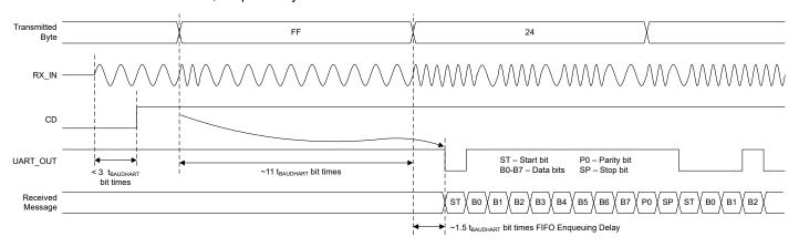
Figure 7-23. HART Receive Start Timing Diagram (SPI and UART Modes)
