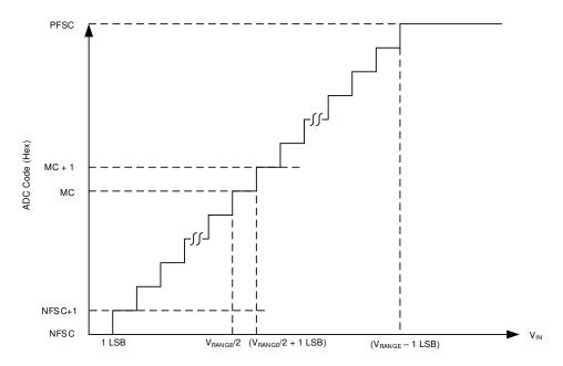
Figure 7-10. ADC Transfer Characteristics
