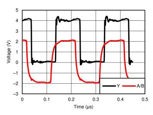
Figure 8-2. Differential 120Ω Terminated Output Waveforms (Cat 5E Cable)
