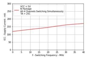
Figure 5-1. Supply Current vs Switching Frequency
