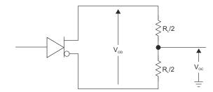
Figure 6-1. Differential and Common-Mode Output Voltages
