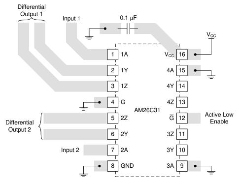
Figure 8-3. Trace Layout on PCB and Recommendations
