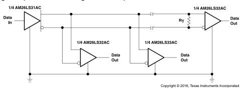
$^{\dagger}R_{T}$  equals the characteristic impedance of the line.
