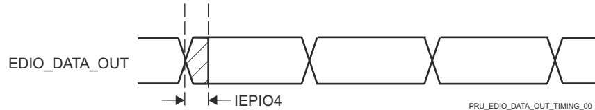
Figure 7-100. PRU_ICSSG IEP Digital IOs Timing Requirements
