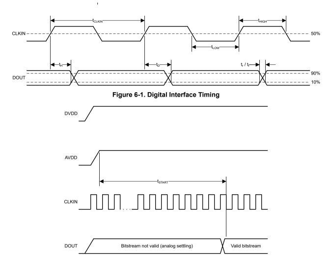
Figure 6-2. Device Start-Up Timing
