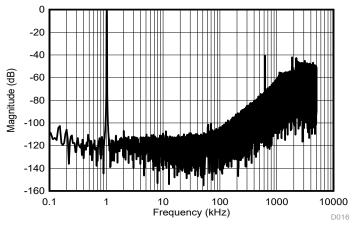
sinc<sup>3</sup> filter, OSR = 2, f<sub>CLKIN</sub> = 20 MHz, f<sub>IN</sub> = 1 kHz
