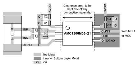
Figure 10-1. Recommended Layout of the AMC1306M05-Q1
