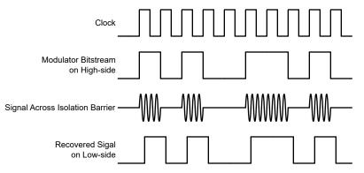
Figure 7-3. OOK-Based Modulation Scheme
