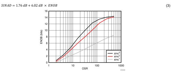
Figure 8-3. Measured Effective Number of Bits vs Oversampling Ratio
