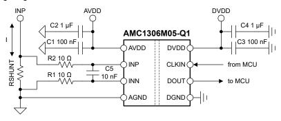
Figure 9-1. Decoupling of the AMC1306M05-Q1
