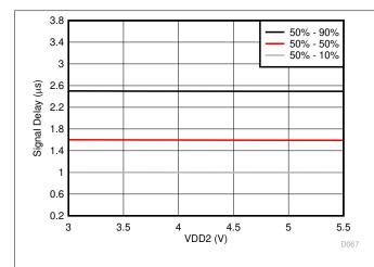
Figure 6-35.  $V_{\text{IN}}$  to  $V_{\text{OUT}}$  Signal Delay vs Low-Side Supply Voltage
