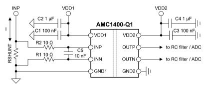
Figure 8-5. Decoupling of the AMC1400-Q1
