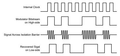
Figure 7-1. OOK-Based Modulation Scheme
