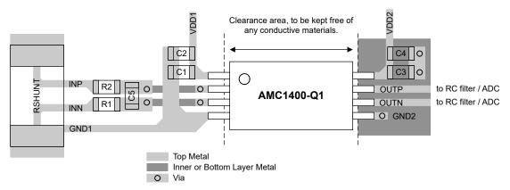
Figure 8-6. Recommended Layout of the AMC1400-Q1
