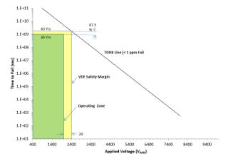
T<sub>A</sub> up to 150°C, stress-voltage frequency = 60 Hz, isolation working voltage = 2000 V<sub>RMS</sub>, operating lifetime = 34 year **Figure 6-4. Reinforced Isolation Capacitor Lifetime Projection**
