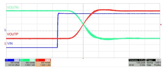
Figure 8-4. Step Response of the AMC1400-Q1
