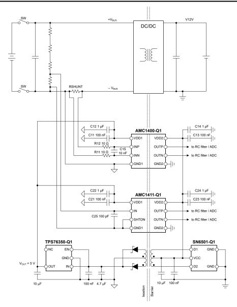
Figure 8-1. Using the AMC1400-Q1 for Current Sensing in a Typical Application
