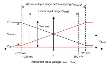
Figure 7-2. Output Behavior of the AMC1400-Q1
