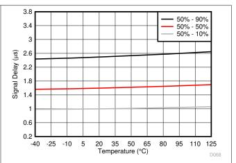
Figure 6-36. V<sub>IN</sub> to V<sub>OUT</sub> Signal Delay vs Temperature
