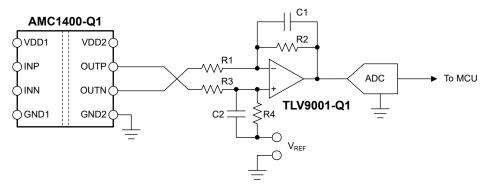
Figure 8-3. Connecting the AMC1400-Q1 Output to a Single-Ended Input ADC
