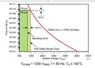
Figure 6-4. Reinforced Isolation Capacitor Lifetime Projection
