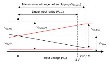
Figure 7-2. Output Behavior of the AMC3311
