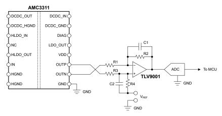
Figure 8-3. Connecting the AMC3311 Output to a Single-Ended Input ADC
