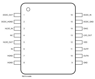
Figure 5-1. DWE Package, 16-Pin SOIC (Top View)
