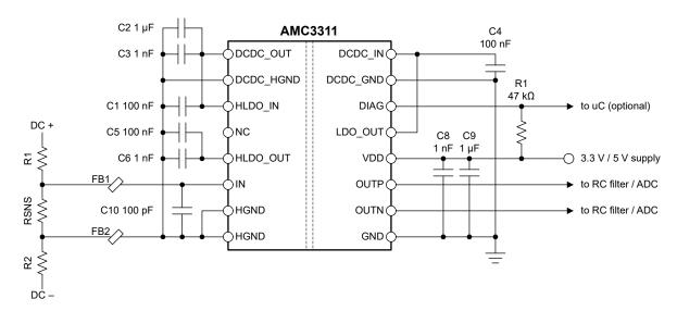
Figure 8-5. Decoupling the AMC3311
