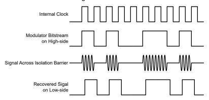
Figure 7-1. OOK-Based Modulation Scheme
