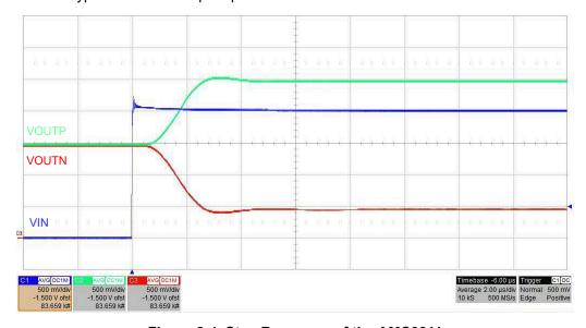
Figure 8-4. Step Response of the AMC3311
