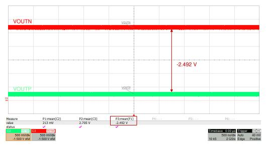
Figure 7-3. Typical Negative Clipping Output of the AMC3311
