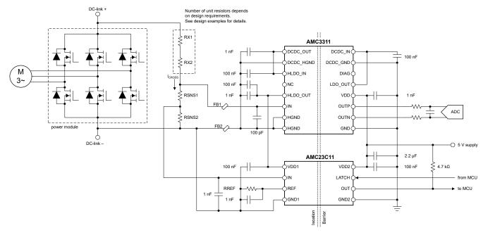
Figure 8-1. The AMC3311 in a Motor Drive Application
