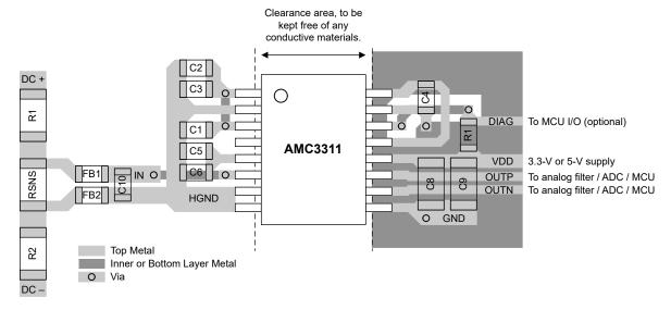
Figure 8-6. Recommended Layout of the AMC3311
