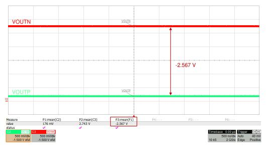
Figure 7-4. Typical Fail-Safe Output of the AMC3311
