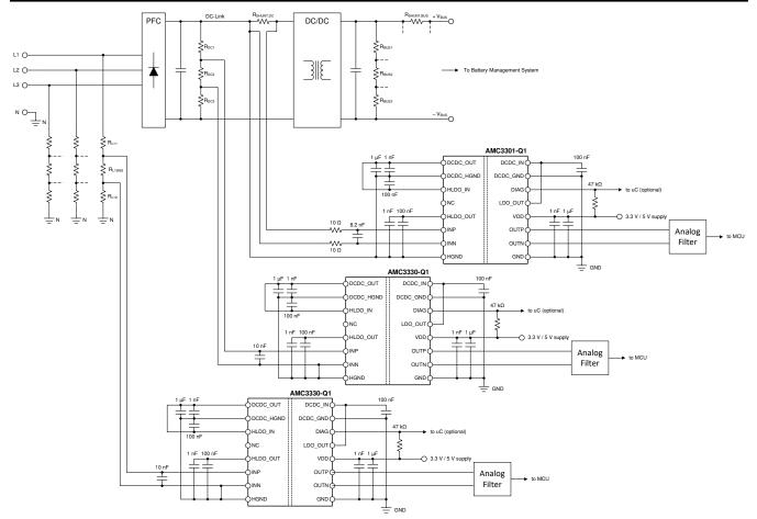
Figure 8-1. The AMC3330-Q1 in an OBC Application
