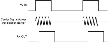
Figure 7-2. OOK-Based Modulation Scheme
