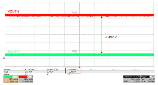
Figure 7-4. Typical Negative Clipping Output of the AMC3330-Q1
