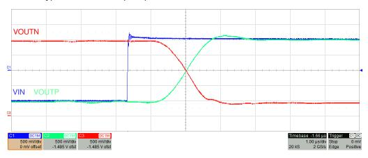
Figure 8-4. Step Respose of the AMC3330-Q1
