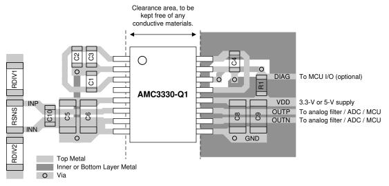
Figure 10-1. Recommended Layout of the AMC3330-Q1
