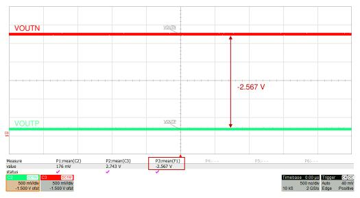
Figure 7-5. Typical Fail-Safe Output of the AMC3330-Q1
