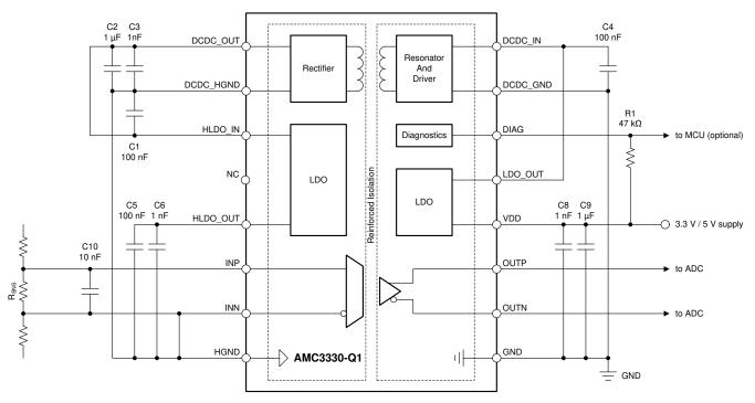
Figure 9-1. Decoupling the AMC3330-Q1
