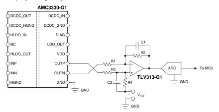
Figure 8-3. Connecting the AMC3330-Q1 Output to a Single-Ended Input ADC
