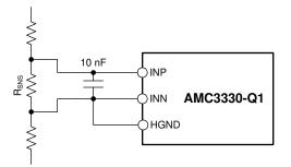
Figure 8-2. Differential Input Filter
