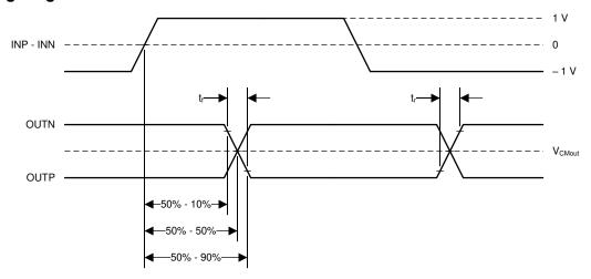
Figure 6-1. Rise, Fall, and Delay Time Waveforms
