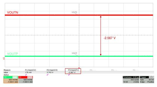
Figure 7-5. Typical Fail-Safe Output of the AMC3330
