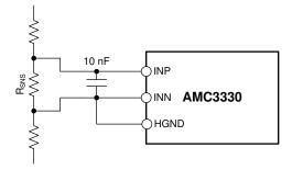
Figure 8-2. Differential Input Filter
