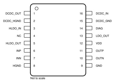
Figure 5-1. DWE Package, 16-Pin SOIC, Top View
