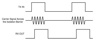
Figure 7-2. OOK-Based Modulation Scheme
