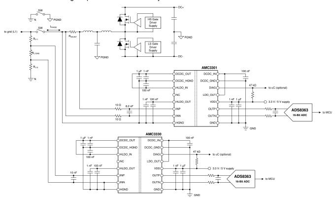
Figure 8-1. The AMC3330 in a Solar Inverter Application
