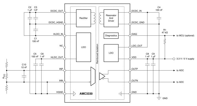
Figure 9-1. Decoupling the AMC3330
