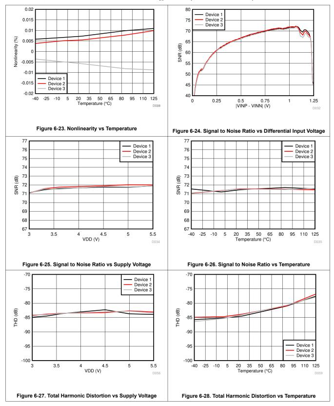
at VDD = 3.3 V, INP = -1 V to 1 V, INN = HGND = 0V, and  $f_{IN}$  = 10 kHz (unless otherwise noted)
