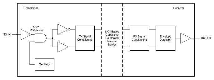
Figure 7-1. Block Diagram of an Isolation Channel
