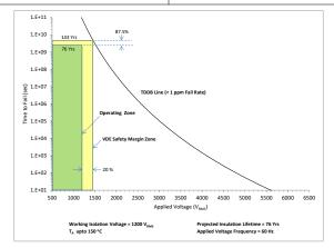
Figure 6-4. Reinforced Isolation Capacitor Lifetime Projection
