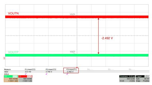
Figure 7-4. Typical Negative Clipping Output of the AMC3330
