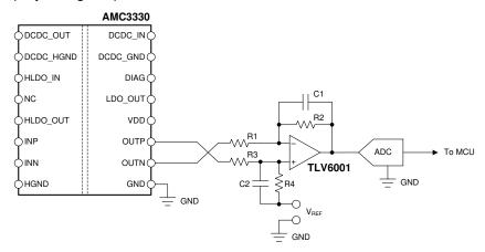
Figure 8-3. Connecting the AMC3330 Output to a Single-Ended Input ADC
