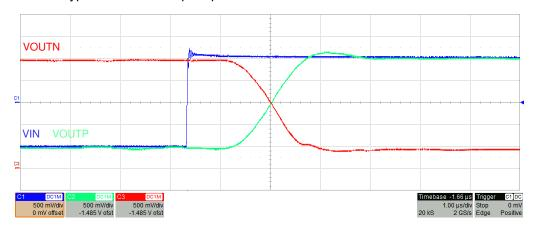
Figure 8-4. Step Respose of the AMC3330
