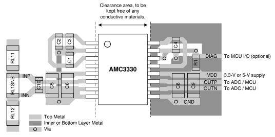
Figure 10-1. Recommended Layout of the AMC3330
