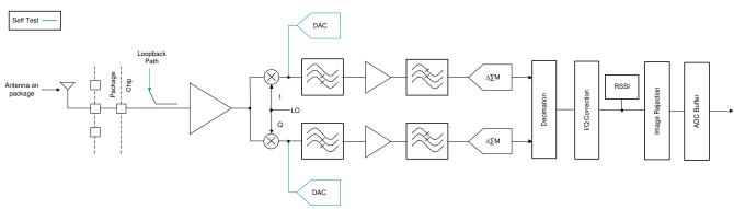
Figure 7-3 describes the receive subsystem.
