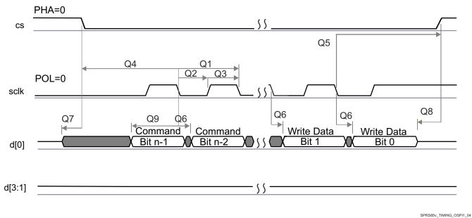
Figure 6-19. QSPI Write (Clock Mode 0)
