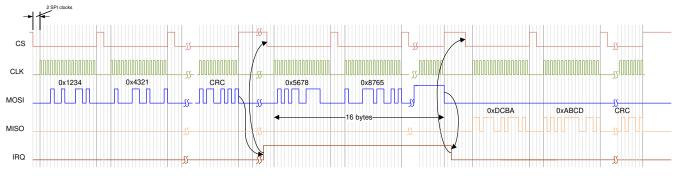
Figure 6-14. SPI Communication
