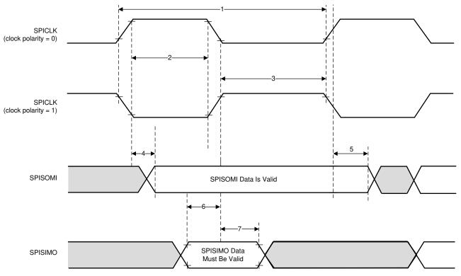
Figure 6-12. SPI Peripheral Mode External Timing (CLOCK PHASE = 0)
