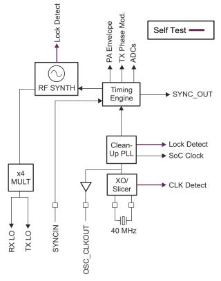
Figure 7-1. Clock Subsystem
