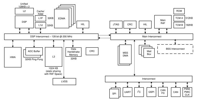
Figure 7-4. Processor Subsystem
