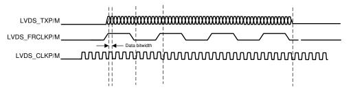
Figure 6-15. LVDS Interface Lane Configuration And Relative Timings
