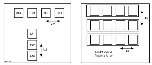
Figure 6-5. Antenna Positions (Placement and Relative Spacing)
