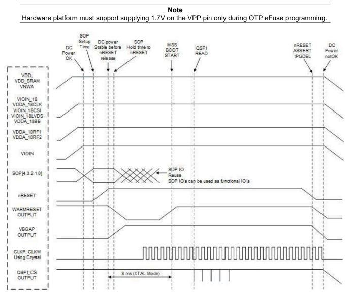
Figure 7-2. Device Wake-up Sequence
