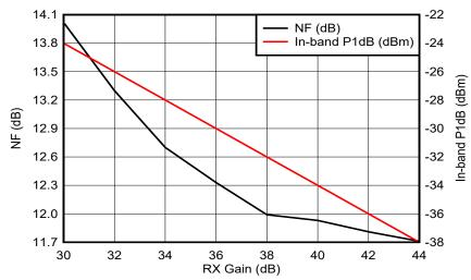
Figure 7-1. Noise Figure, In-band P1dB vs Receiver Gain (TBD)
