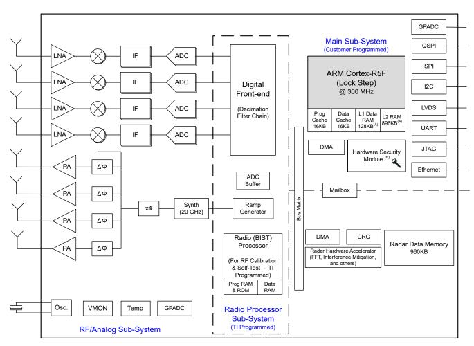
Figure 8-1. Functional Block Diagram
