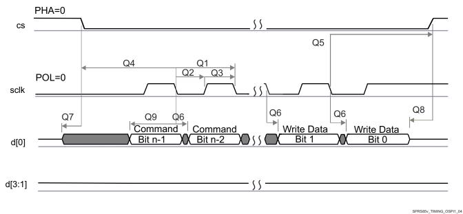
Figure 7-5. QSPI Write (Clock Mode 0)
