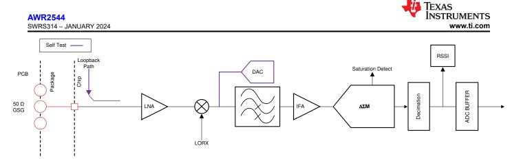
Figure 8-4. Receive Subsystem (Per Channel)
