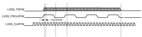
Figure 7-21. LVDS Interface Lane Configuration And Relative Timings
