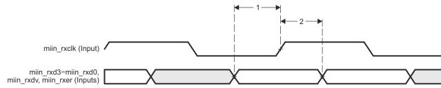
Figure 7-18. MAC Receive Interface Timing, MIIn operation
