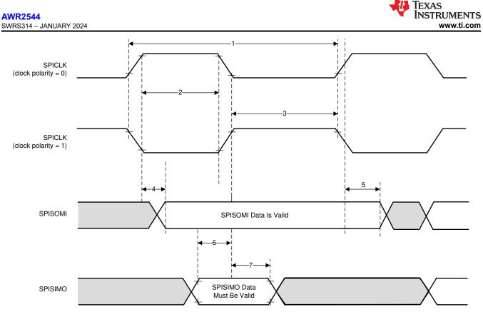
Figure 7-10. SPI Peripheral Mode External Timing (CLOCK PHASE = 0)
