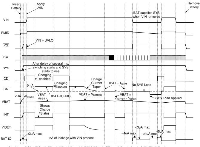
Conditions: PGB\_MRS = 0, TE = 1, SW\_LDO = 1, VINDPM\_ON = 0, PG and INT pulled up to SYS, EN\_INT = 1
