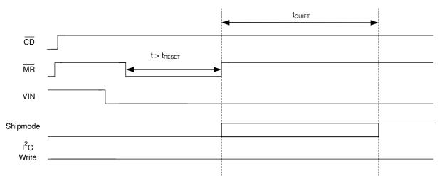
Figure 9-2. CD, MR and VIN Sequencing for Ship Mode Entry Through Long MR button press
