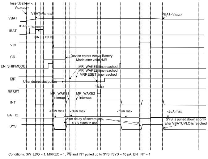
Figure 8-2. Battery Operation and Sleep Mode
