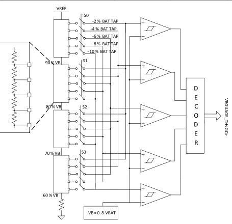
Figure 9-3. Voltage Battery Monitor
