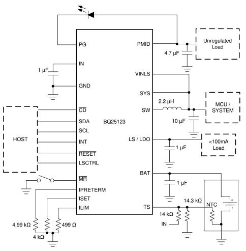
Figure 10-1. Typical Application Circuit
