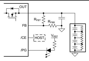
Figure 7-2. BQ25173-Q1 Feedback Divider
