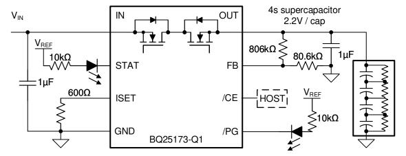
Figure 8-11. BQ25173-Q1 4s Supercapacitor Application Diagram
