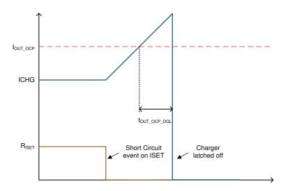
Figure 7-3. Overcurrent Protection
