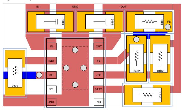
Figure 10-1. BQ25173-Q1 Board Layout Example
