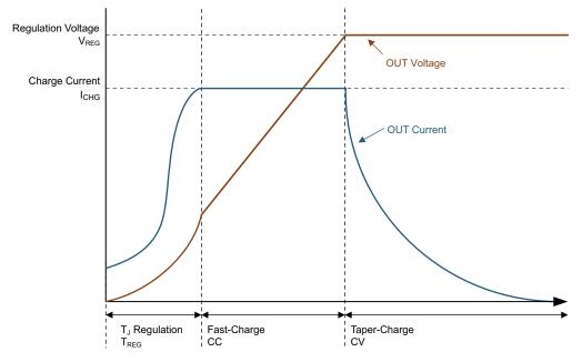
Figure 7-1. Supercapacitor Charging Profile with Thermal Regulation
