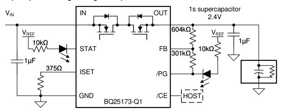
Figure 8-1. BQ25173-Q1 1s Supercapacitor Application Diagram
