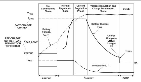
Figure 7-1. Lithium-Ion Battery Charging Profile with Thermal Regulation
