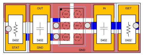
Figure 10-1. BQ25175 Board Layout Example
