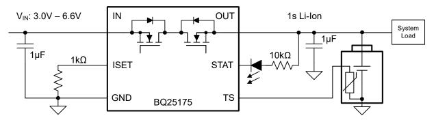
Figure 8-1. BQ25175 Typical Application for 1s Li-lon Charging at 100 mA
