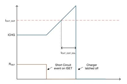
Figure 7-4. Overcurrent Protection
