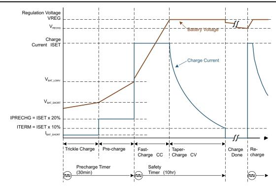
Figure 7-2. Battery Charging Profile
