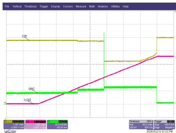
Figure 8-9. ISET Short-Circuit Response
