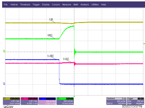
Figure 8-7. OUT Transient Response
