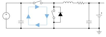
Figure 12-1. High Frequency Current Path
