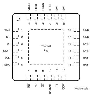
Figure 7-1. RTW Package 24-Pin WQFN Top View
