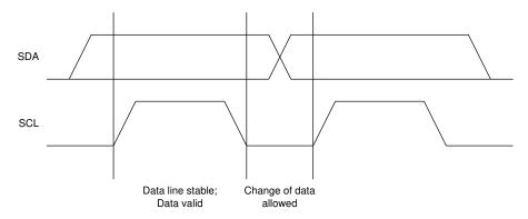
Figure 9-8. Bit Transfer on the I<sup>2</sup>C Bus
