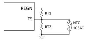
Figure 9-6. TS Pin Resistor Network
