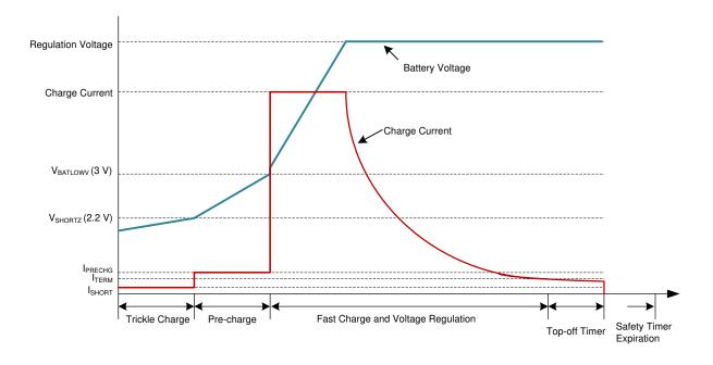
Figure 9-4. Battery Charging Profile
