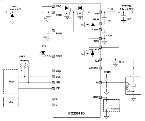
Figure 10-1. BQ25611D Application Diagram
