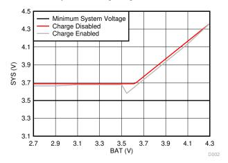
Figure 9-1. System Voltage vs Battery Voltage
