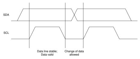
Figure 9-6. Bit Transfer on the I<sup>2</sup>C Bus
