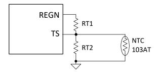
Figure 9-4. TS Pin Resistor Network
