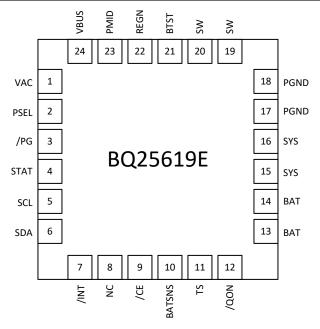
Figure 7-2. BQ25619E RTW Package 24-Pin WQFN Top View
