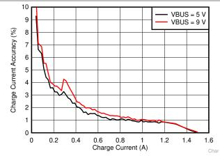
Figure 8-3. Charge Current Accuracy
