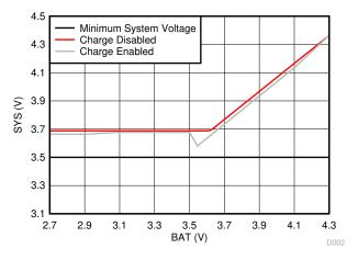
Figure 9-1. System Voltage vs Battery Voltage
