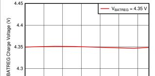
Figure 8-4. Battery Charge Voltage vs Junction Temperature
