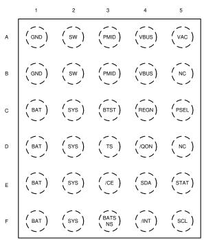
Figure 7-1. BQ25618E YFF Package 30-Pin WCSP Top View
