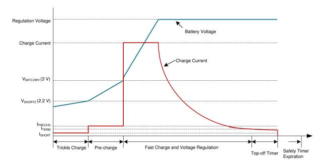
Figure 9-2. Battery Charging Profile
