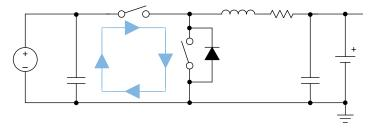
Figure 12-1. High Frequency Current Path
