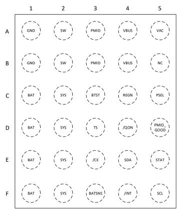
Figure 6-1. BQ25618 YFF Package 30-Pin WCSP Top View
