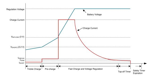
Figure 8-3. Battery Charging Profile
