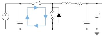
Figure 11-1. High Frequency Current Path
