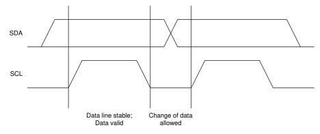
Figure 8-7. Bit Transfer on the I<sup>2</sup>C Bus
