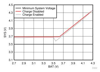
Figure 8-1. System Voltage vs Battery Voltage
