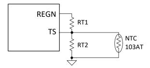
Figure 8-5. TS Pin Resistor Network
