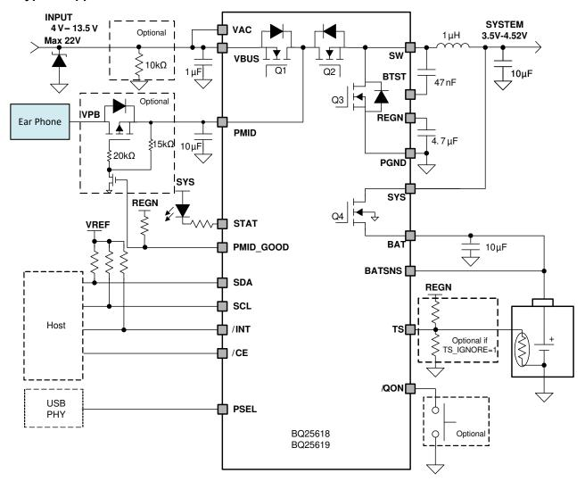
Figure 9-1. BQ25619 Application Diagram with Optional PMOS
