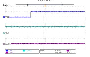
VAC1 connected to input source 1, VBUS connected to input source 2, VAC2 short to VBUS, ACDRV1 active, ACDRV2 short to ground
