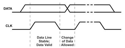
Figure 8-11. Bit Transfer on the Serial Interface
