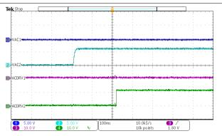
VAC1 connected to input source 1, VAC2 connected to input source 2, ACDRV1 and ACumDRV2 active
