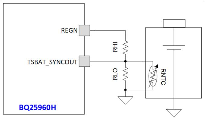
Figure 8-8. TSBAT\_SYNCOUT Resistor Network
