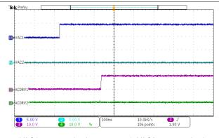
VAC1 connected to input source 1, VAC2 connected to input source 2, ACDRV1 and ACDRV2 active
