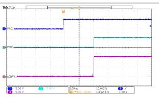
VAC1 connected to input source, VAC2 short to VBUS, ACDRV1 active, ACDRV2 short to ground
