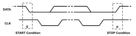
Figure 8-10. START and STOP Condition
