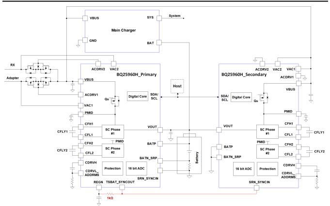
Figure 8-9. Parallel Operation of BQ25960H
