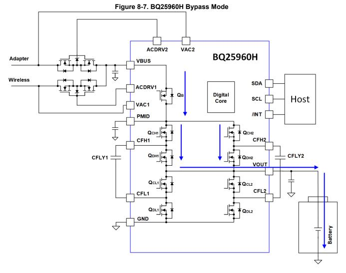
To change from Bypass Mode to Switched Cap Mode or from Switched Cap to Bypass Mode, the host would first set CHG\_EN=0 to stop the converter and then set EN\_BYPASS to desired value. The host sets desired protection threshold based on the selected operation modes and then host enables charge by setting CHG\_EN=1.
