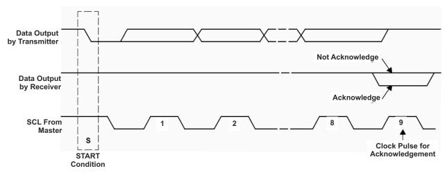
Figure 8-12. Acknowledge on the I<sup>2</sup>C BUS
