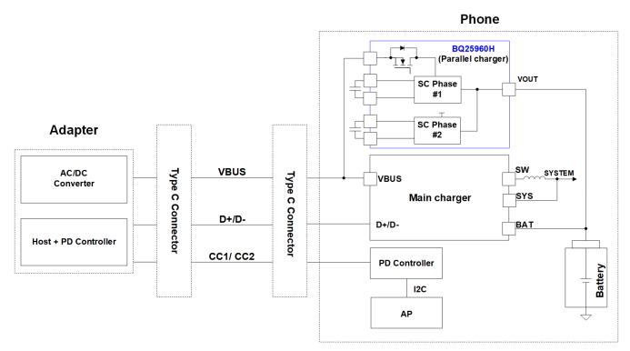
Figure 8-1. BQ25960H System Diagram
