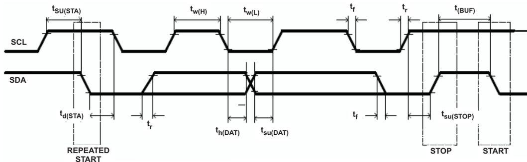
Figure 1. I<sup>2</sup>C-Compatible Interface Timing Diagrams
