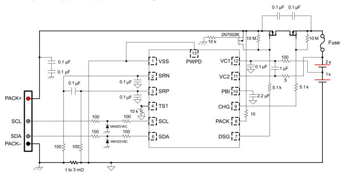
Note: The input filter capacitors of 0.1  $\mu\text{F}$  for the SRN and SRP pins must be located near the pins of the device.
