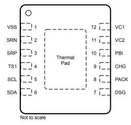
Figure 6-1. DRZ Package 12-Pin VSON Top View
