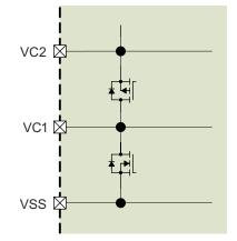
Figure 8-3. Internal Cell Balancing
