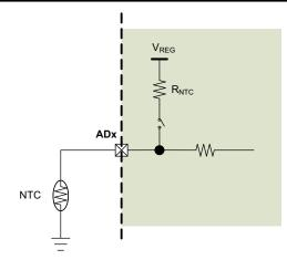
Figure 8-1. External Thermistor Biasing
