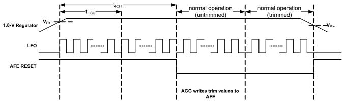
Figure 8-2. POR Timing Diagram
