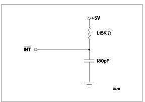
Figure 4. Output Load A
