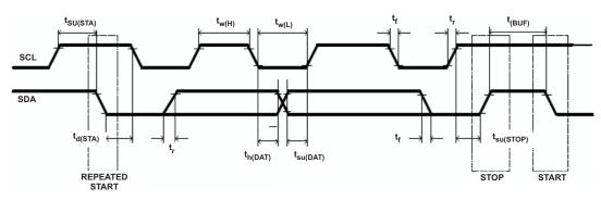
Figure 1. I<sup>2</sup>C-Compatible Interface Timing Diagrams
