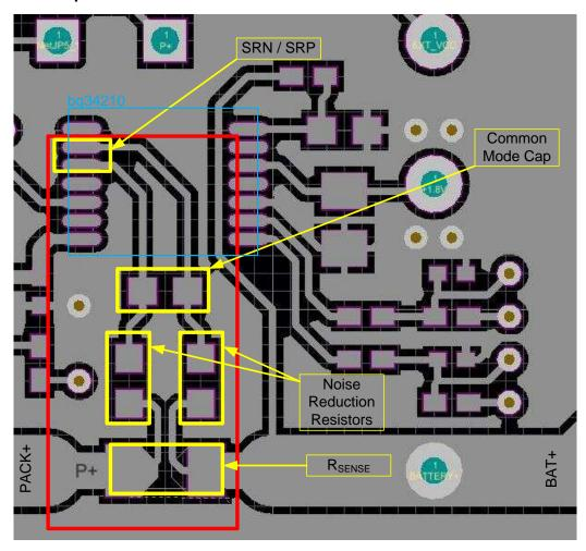
Figure 8. bq34210-Q1 Sense Resistor Layout
