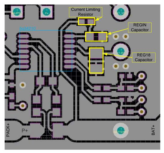
Figure 9. bq34210-Q1 Capacitor Layout
