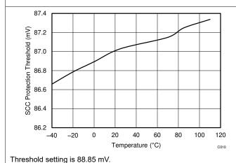
Figure 7-8. Short Circuit Charge Protection
