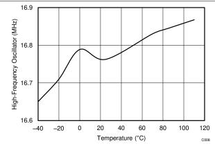
Figure 7-6. High-Frequency Oscillator vs. Temperature
