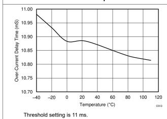
Figure 9-21. Overcurrent Delay Time vs. Temperature
