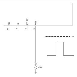
Figure 9-8. System Present Pull-Down Resistor
