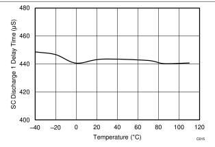
Threshold setting is 465  $\mu s$  (including internal delay).
