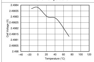
Figure 7-14. V<sub>CELL</sub> Measurement at 2.5-V vs. Temperature
