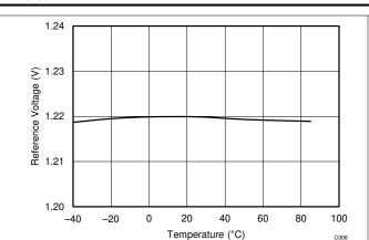
Figure 7-4. Reference Voltage vs. Temperature
