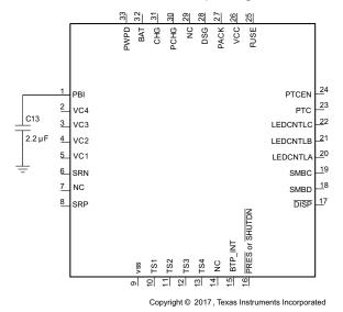
Figure 9-7. Power Supply Decoupling
