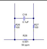
Figure 9-6. Differential Filter
