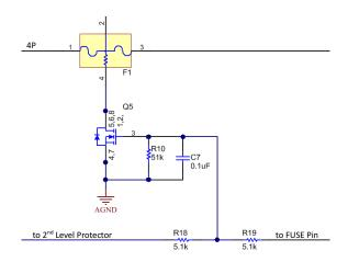
Figure 9-3. FUSE Circuit
