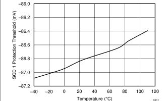
Figure 7-7. Overcurrent Discharge Protection Threshold vs. Temperature
