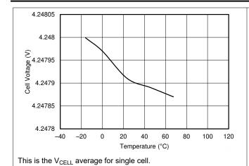
Figure 7-16.  $V_{CELL}$  Measurement at 4.25-V vs. Temperature
