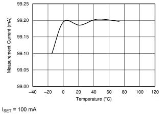
Figure 7-17. I measured vs. Temperature
