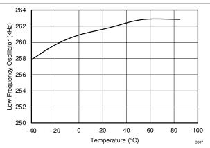
Figure 7-5. Low-Frequency Oscillator vs. Temperature
