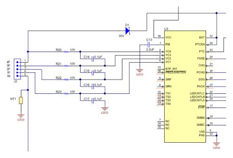
Figure 9-12. Cell and BAT Inputs
