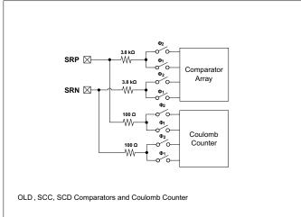
Figure 6-3. Pin Equivalent Diagram 3
