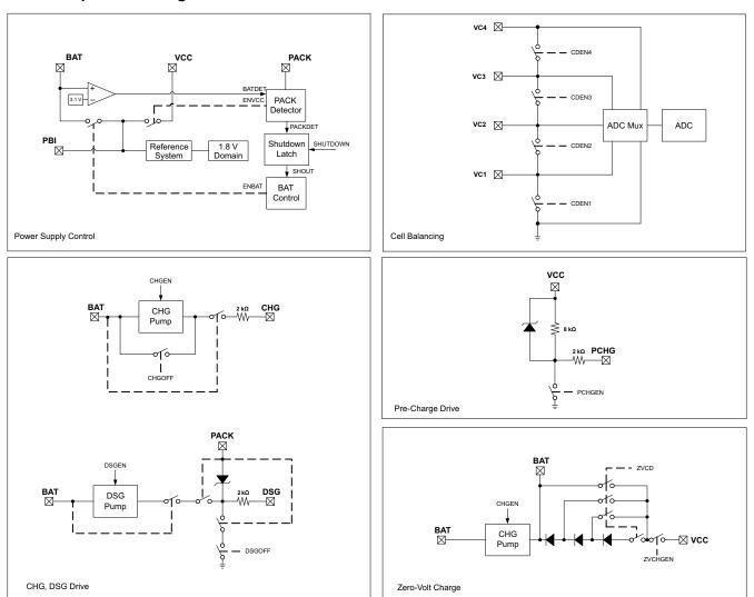
Figure 6-1. Pin Equivalent Diagram 1
