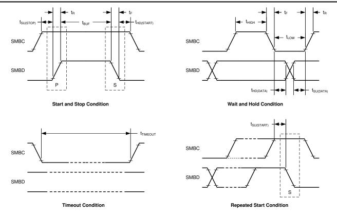
Figure 7-1. SMBus Timing Diagram
