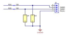
Figure 9-10. ESD Protection for SMBus Communication
