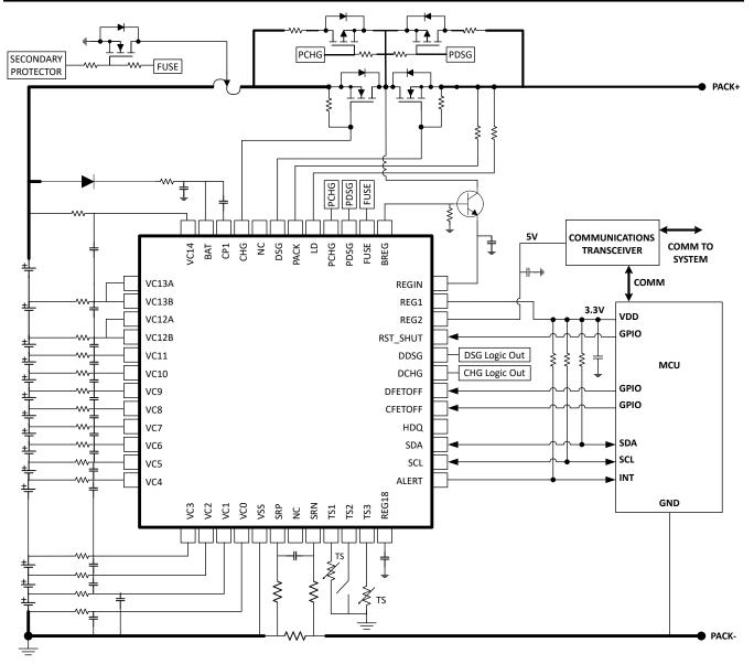
Figure 16-1. BQ769142 14-Series Cell Typical Implementation (Simplified Schematic)
