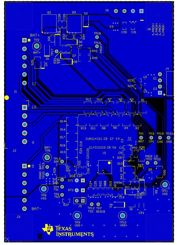
Figure 18-2. BQ76952 Two-Layer Board Layout–Bottom Layer
