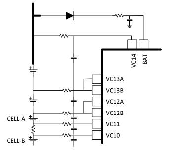
Figure 10-1. Using Cell Input Pins for Interconnect Measurement
