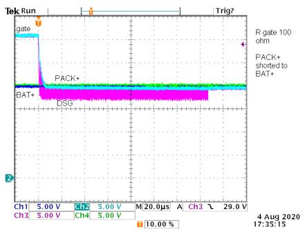
Figure 16-9. A Fast Turn-Off Case with a 100- $\Omega$  Series Gate Resistor
