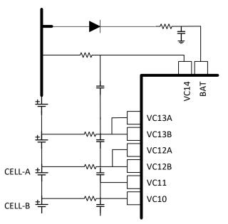
Figure 10-2. Terminating an Unused Cell Input Pin
