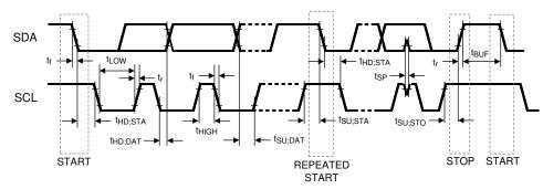
Figure 7-1. I<sup>2</sup>C Communications Interface Timing
