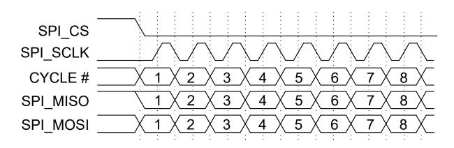
Figure 14-4. SPI with CPOL = 0 and CPHA = 0
