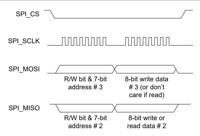
Figure 14-10. SPI Transaction #3 Without CRC
