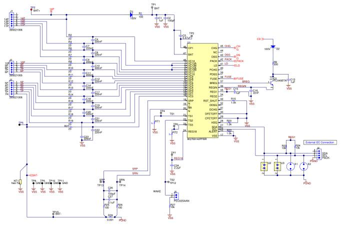
Figure 16-2. BQ769142 14-Series Cell Schematic Diagram—Monitor
