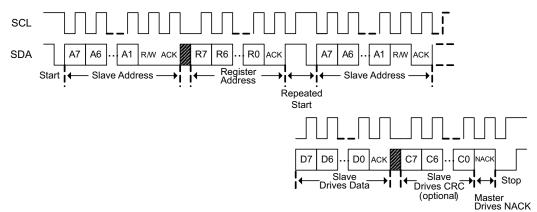
Figure 14-2. I<sup>2</sup>C Read with Repeated Start
