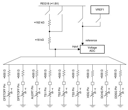
Figure 10-3. External Thermistor Biasing
