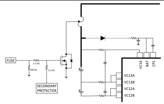
Figure 12-1. FUSE Pin Operation
