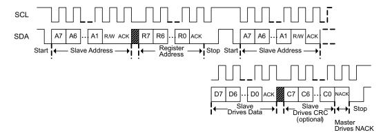
Figure 14-3. I<sup>2</sup>C Read Without Repeated Start
