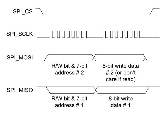
Figure 14-9. SPI Transaction #2 Without CRC
