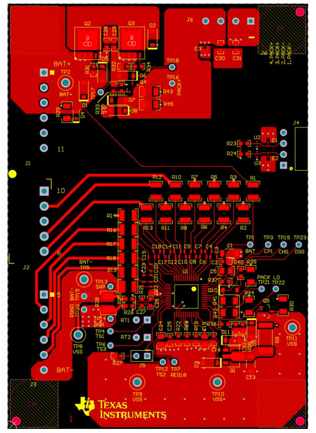
Figure 18-1. BQ76952 Two-Layer Board Layout–Top Layer
