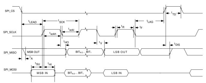
Figure 7-2. SPI Communications Interface Timing
