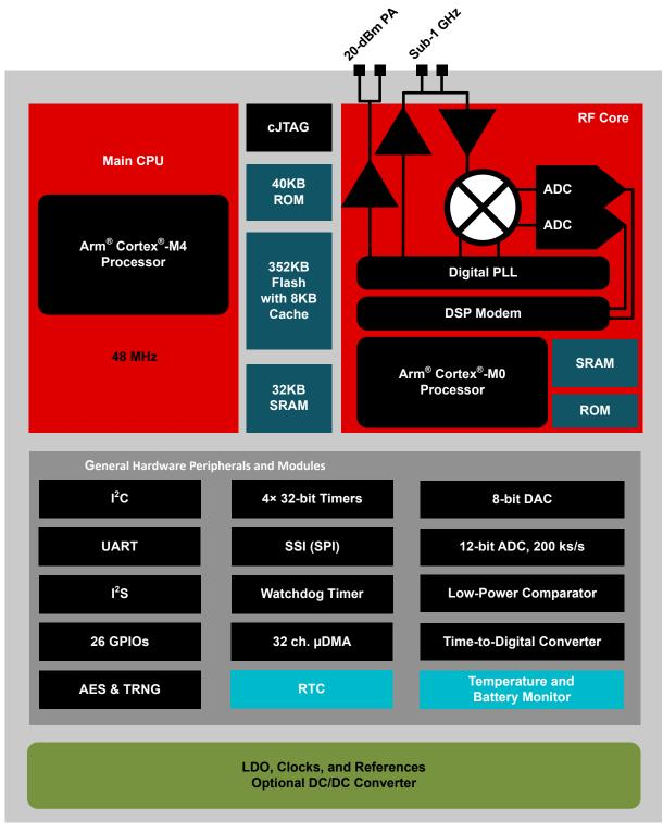
Figure 4-1. CC1311P3 Functional Block Diagram
