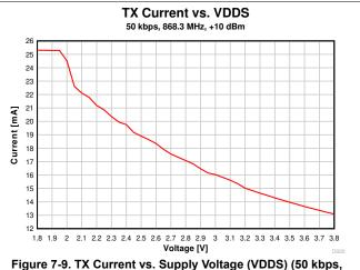
Figure 7-9. TX Current vs. Supply Voltage (VDDS) (50 kbps; 868.3 MHz)
