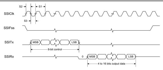
Figure 7-2. SSI Timing for MICROWIRE Frame Format (FRF = 10), Single Transfer
