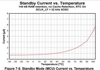
Figure 7-5. Standby Mode (MCU) Current vs. Temperature
