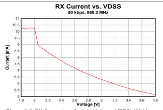
Figure 7-7. RX Current vs. Supply Voltage (VDDS) (50 kbps, 868.3 MHz)
