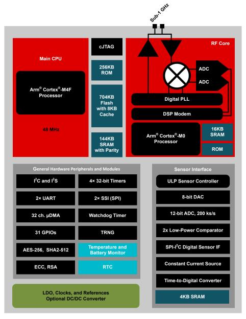
Figure 3-1. CC1312R7 Block Diagram
