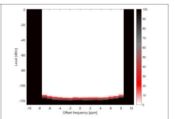
Figure 7-17. Narrowband, 9.6 kbps ±2.4 kHz deviation, 2-GFSK, 868 MHz, 17.1 kHz RX Bandwidth
