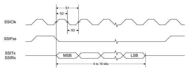
Figure 7-1. SSI Timing for TI Frame Format (FRF = 01), Single Transfer Timing Measurement
