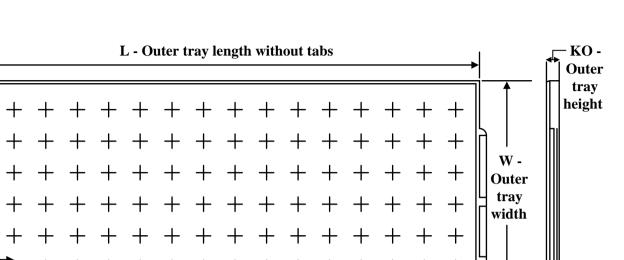
P1 - Tray unit pocket pitch CW - Measurement for tray edge (Y direction) to corner pocket center CL - Measurement for tray edge (X direction) to corner pocket center
