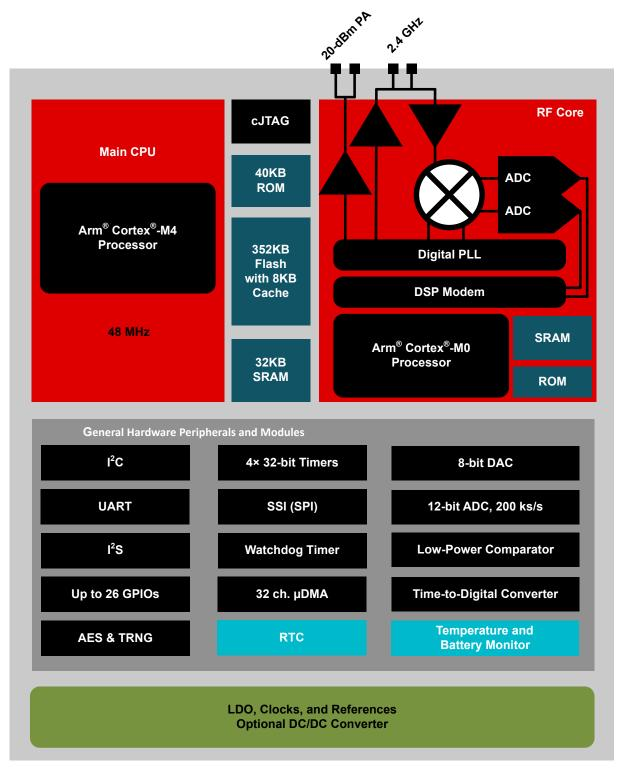
Figure 4-1. CC2651P3 Functional Block Diagram
