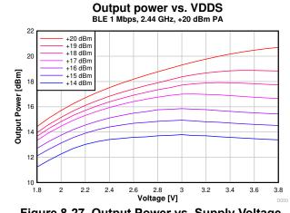
Figure 8-27. Output Power vs. Supply Voltage (VDDS) (BLE 1 Mbps, 2.44 GHz, +20 dBm PA)
