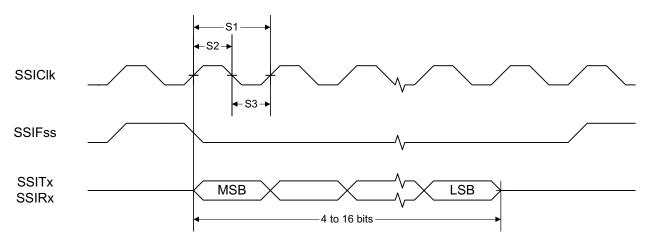
Figure 8-1. SSI Timing for TI Frame Format (FRF = 01), Single Transfer Timing Measurement
