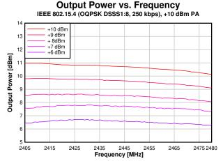
Figure 8-32. Output Power vs. Frequency (250 kbps, +10 dBm PA)
