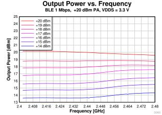
Figure 8-31. Output Power vs. Frequency (BLE 1 Mbps, 2.44 GHz, +20 dBm PA)
