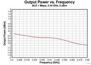
Figure 8-29. Output Power vs. Frequency (BLE 1 Mbps, 2.44 GHz)
