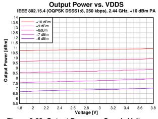
Figure 8-28. Output Power vs. Supply Voltage (VDDS) (2.44 GHz, +10 dBm PA)
