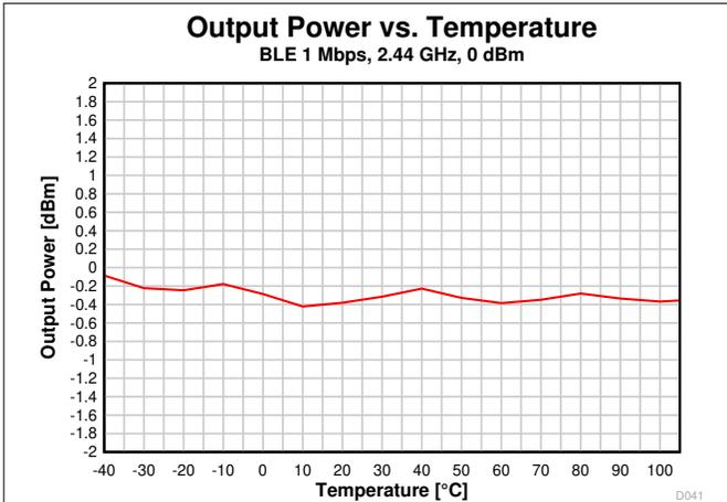
Figure 8-17. Output Power vs. Temperature (BLE 1 Mbps, 2.44 GHz)
