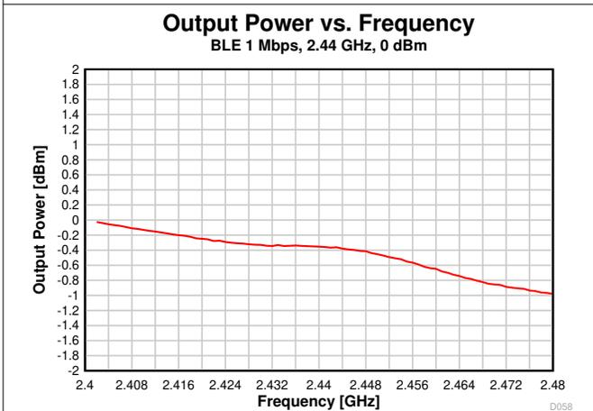
Figure 8-21. Output Power vs. Frequency (BLE 1 Mbps, 2.44 GHz)
