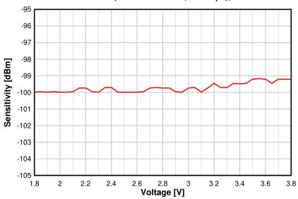
Figure 8-17. Sensitivity vs. Supply Voltage (VDDS) IEEE 802.15.4 (OQPSK DSSS1:8, 250 kbps)
