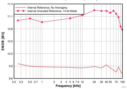
Figure 8-25. ENOB vs. **Input Frequency**
