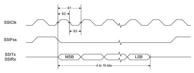
Figure 8-1. SSI Timing for TI Frame Format (FRF = 01), Single Transfer Timing Measurement
