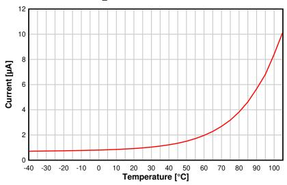
Figure 8-6. Standby Mode (MCU) Current vs.
