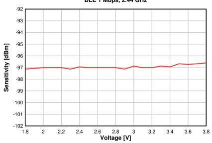
Figure 8-15. Sensitivity vs. Supply Voltage (VDDS) (BLE 1 Mbps, 2.44 GHz)
