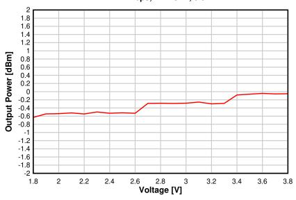
Figure 8-20. Output Power vs. Supply Voltage (VDDS) (BLE 1 Mbps, 2.44 GHz, 0 dBm)
