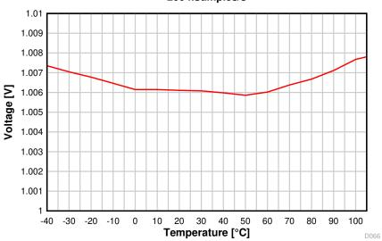
Figure 8-29. ADC Accuracy vs. Temperature
