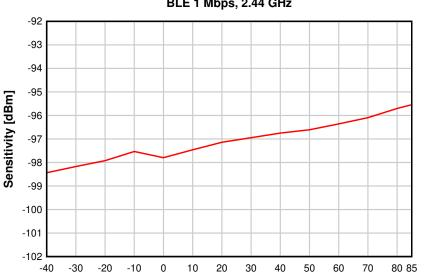
Figure 8-13. Sensitivity vs. Temperature (BLE 1 Mbps, 2.44 GHz)
