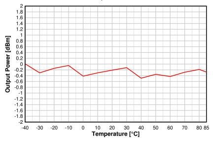
Figure 8-18. Output Power vs. Temperature (BLE 1 Mbps, 2.44 GHz, 0 dBm)
