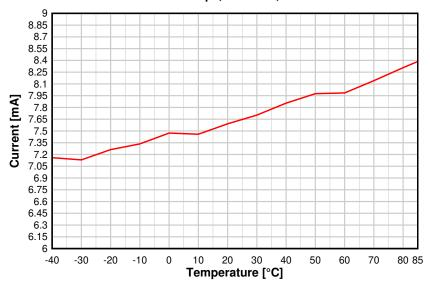
Figure 8-9. TX Current vs. Temperature (BLE 1 Mbps, 2.44 GHz)
