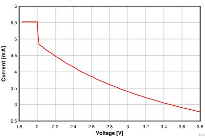
Figure 8-4. Active Mode (MCU) Current vs. Supply Voltage (VDDS)
