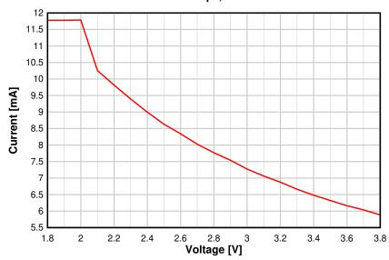
Figure 8-8. RX Current vs. Supply Voltage (VDDS) (BLE 1 Mbps, 2.44 GHz)
