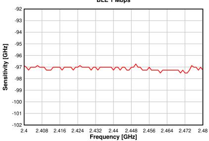
Figure 8-11. Sensitivity vs. Frequency (BLE 1 Mbps, 2.44 GHz)
