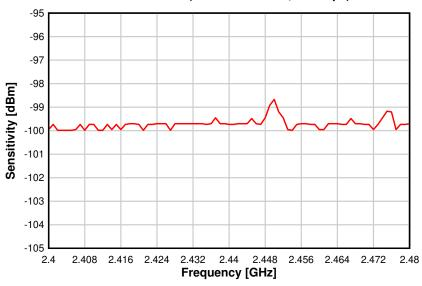
Figure 8-12. Sensitivity vs. Frequency IEEE 802.15.4 (OQPSK DSSS1:8, 250 kbps)
