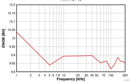
Figure 8-26. ENOB vs. **Sampling Frequency**
