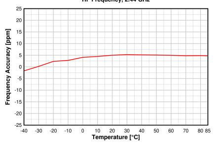
Figure 8-24. Compensated Frequency Accuracy vs. Temperature (2.44 GHz)
