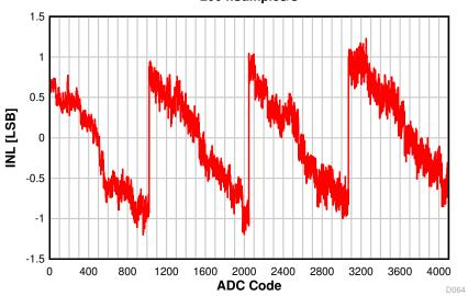
Figure 8-27. INL vs. ADC Code
