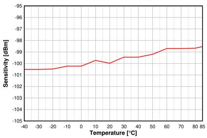
Figure 8-14. Sensitivity vs. Temperature IEEE 802.15.4 (OQPSK DSSS1:8, 250 kbps)
