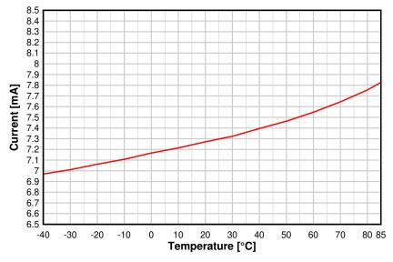
Figure 8-7. RX Current vs. Temperature (BLE 1 Mbps, 2.44 GHz)
