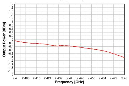
Figure 8-22. Output Power vs. Frequency (BLE 1 Mbps, 2.44 GHz, 0 dBm)
