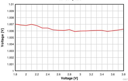
Figure 8-30. ADC Accuracy vs. Supply Voltage (VDDS)
