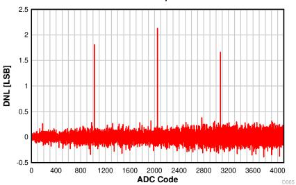
Figure 8-28. DNL vs. ADC Code
